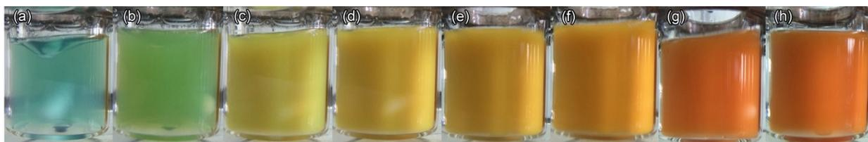
**Fig. S9** Photographs showing the color change of the solution as a function of reaction time during synthesis of  $\text{Cu}_2\text{O}$  cubic nanocrystals in Fig. 3b. (a) 5 s, (b) 10 s, (c) 15 s, (d) 20 s, (e) 30 s, (f) 60 s, (g) 5 min, and (h) 60 min after adding sodium ascorbate.
