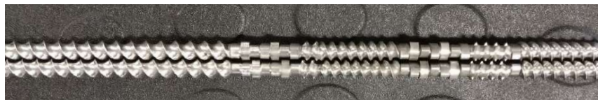
Figure S2. Steel twin-screw set configuration employed in the oligomerisation of the amino acids (12 mm in diameter, 40 cm in length).
