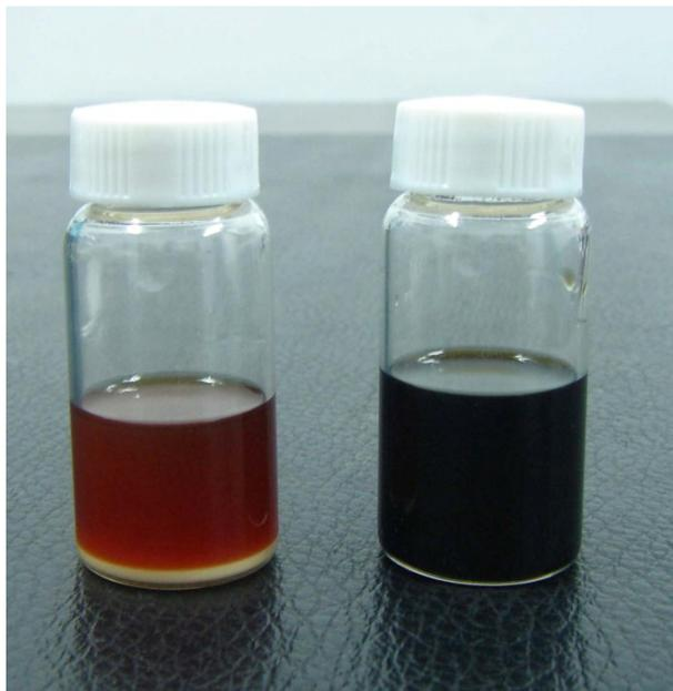
**Figure S7.** Glucose conversion to 5-HMF over SPPS (left) and  $\text{CrCl}_2$  (right) in ionic liquid solvent (Reaction condition: 0.18 g catalyst, solvent 20 ml, 140 °C for 1 h, glucose 1.8 g)
