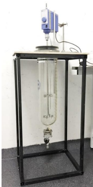
Figure S2. The reactor used in large scale CLP formation.
