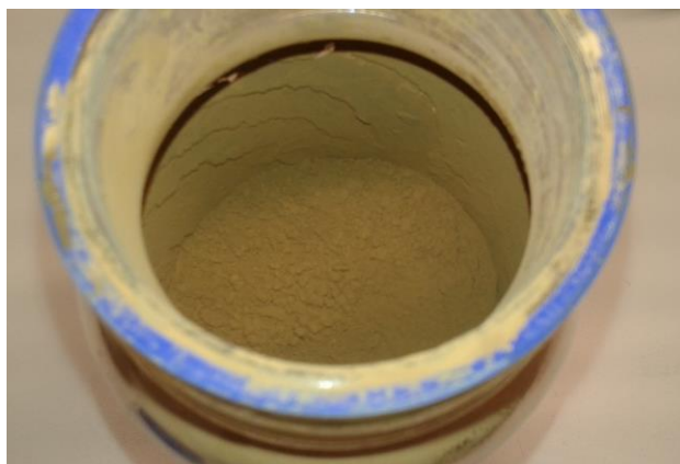
Figure S5. Spray dried CLP powder.
