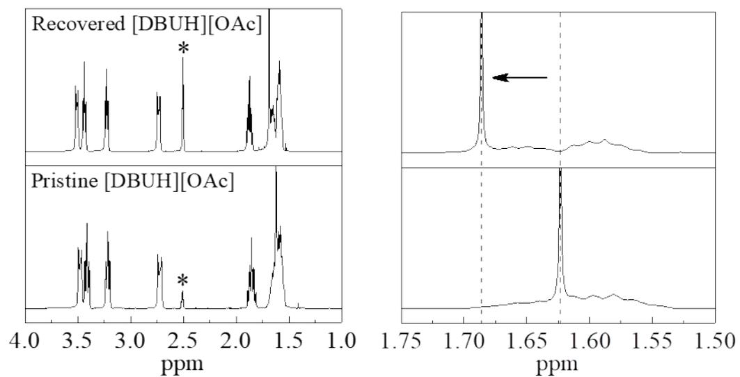
Figure S6 (a)  $^1\text{H}$  NMR spectra of recovered [DBUH][OAc] by the distillation under reduced pressure at 190 °C and the pristine one in  $\text{DMSO-}d_6$  (\*solvent) and (b) enlarged  $^1\text{H}$  NMR spectra in the range of 1.50 and 1.75 ppm.
