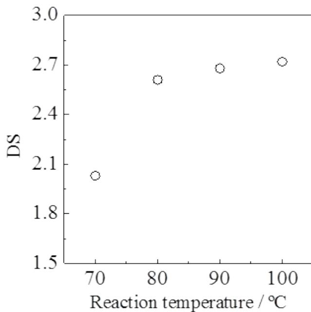
Figure S4 Effect of acetylation temperature on DS values in [DBUH][OAc] (acetylation time: 24 h, cellulose: 5 wt%, Ac<sub>2</sub>O: 3 equivalent to AGU).
