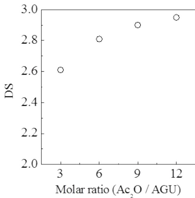
Figure S5 Effect of Ac<sub>2</sub>O-to-AGU molar ratio on DS values in [DBUH][OAc] (acetylation temperature: 80 °C, acetylation time: 24 h, cellulose: 5 wt%).
