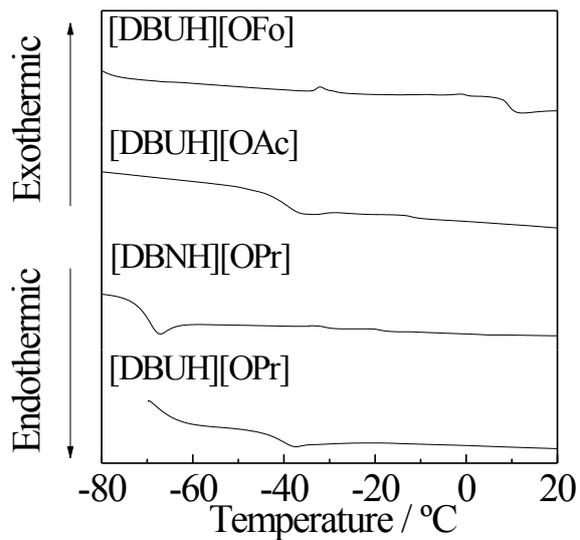
Figure S3 Expanded DSC curves of [DBUH][OFo], [DBUH][OAc], [DBNH][OPr], and [DBUH][OPr] (from -80 to 20 °C).
