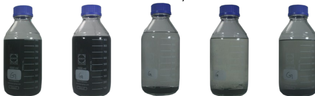
Figure S10. Stability of chlorophyll extracts-assisted exfoliated graphene in solvents. Stable homogeneous suspensions of chlorophyll-assisted exfoliated graphene in various solvents after five days, from left to right: tetrahydrofuran, ethyl acetate, ethanol, hexane, and toluene.
