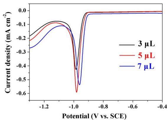
**Fig. S9** Linear sweep voltammograms of 3  $\mu\text{L}$ , 5  $\mu\text{L}$  and 7  $\mu\text{L}$  of 1  $\text{mg mL}^{-1}$  hollow urchin-like  $\text{Co}(\text{CO}_3)_{0.5}(\text{OH})\cdot 0.11\text{H}_2\text{O}$  in  $\text{CO}_2$ -saturated 0.1 M  $\text{NaHCO}_3$  aqueous solution (scan rate of 20  $\text{mV s}^{-1}$ ).
