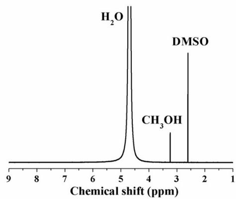
**Fig. S4**  $^1\text{H}$ -NMR spectra of the electrolyte after  $\text{CO}_2$  reduction electrolysis at  $-0.98$  V (vs. SCE) for 10 h at Cu electrode.
