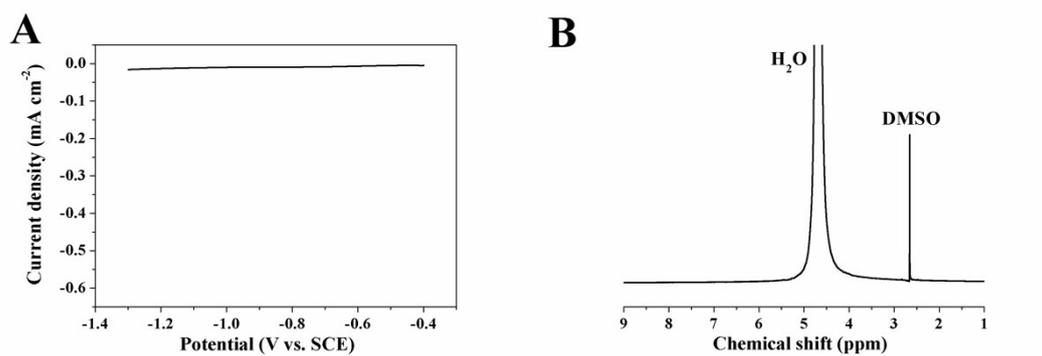
**Fig. S6** (A) Linear sweep voltammogram of bare glassy carbon electrode with Nafion film in CO<sub>2</sub>-saturated 0.1 M NaHCO<sub>3</sub> aqueous solution (scan rate of 20 mV s<sup>-1</sup>). (B) <sup>1</sup>H-NMR spectra of the electrolyte after CO<sub>2</sub> reduction electrolysis at -0.98 V (vs. SCE) for 10 h at bare glassy carbon electrode with Nafion film.
