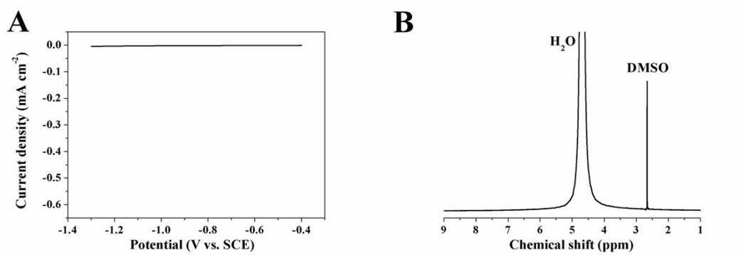
**Fig. S5** (A) Linear sweep voltammogram of bare glassy carbon electrode in CO<sub>2</sub>-saturated 0.1 M NaHCO<sub>3</sub> aqueous solution (scan rate of 20 mV s<sup>-1</sup>). (B) <sup>1</sup>H-NMR spectra of the electrolyte after CO<sub>2</sub> reduction electrolysis at -0.98 V (vs. SCE) for 10 h at bare glassy carbon electrode.
