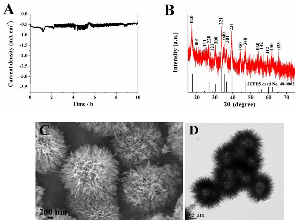
**Fig. S10** (A) Constant-potential electrolysis at  $-0.98 \text{ V}$  (vs. SCE) for 10 h in  $0.1 \text{ M NaHCO}_3$  aqueous solution with  $\text{CO}_2$  flow at the hollow urchin-like  $\text{Co}(\text{CO}_3)_{0.5}(\text{OH}) \cdot 0.11\text{H}_2\text{O}$ . (B) XRD pattern, (C) SEM image and (D) TEM image of hollow urchin-like  $\text{Co}(\text{CO}_3)_{0.5}(\text{OH}) \cdot 0.11\text{H}_2\text{O}$  electrocatalyst after 10 h electrolysis.
