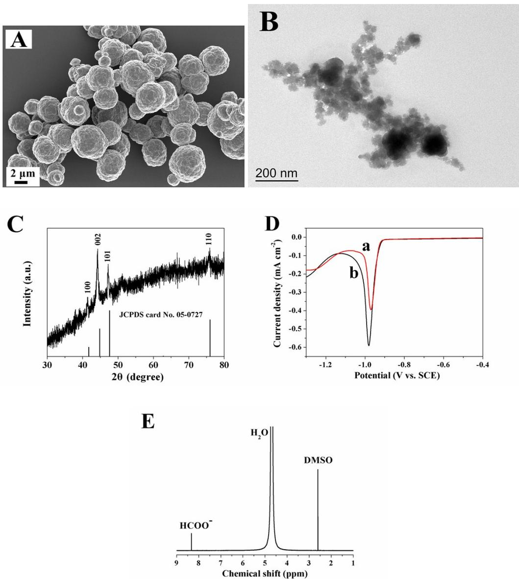
**Fig. S2** (A) SEM image, (B) TEM image and (C) XRD pattern of Co sphere. (D) Linear sweep voltammograms of (a) Co sphere and (b) hollow urchin-like  $\text{Co}(\text{CO}_3)_{0.5}(\text{OH}) \cdot 0.11\text{H}_2\text{O}$  in  $\text{CO}_2$ -saturated 0.1 M  $\text{NaHCO}_3$  aqueous solution (scan rate of  $20 \text{ mV s}^{-1}$ ). (E)  $^1\text{H}$ -NMR spectra of the electrolyte after  $\text{CO}_2$  reduction electrolysis at  $-0.98 \text{ V}$  (vs. SCE) for 10 h at the Co sphere.
