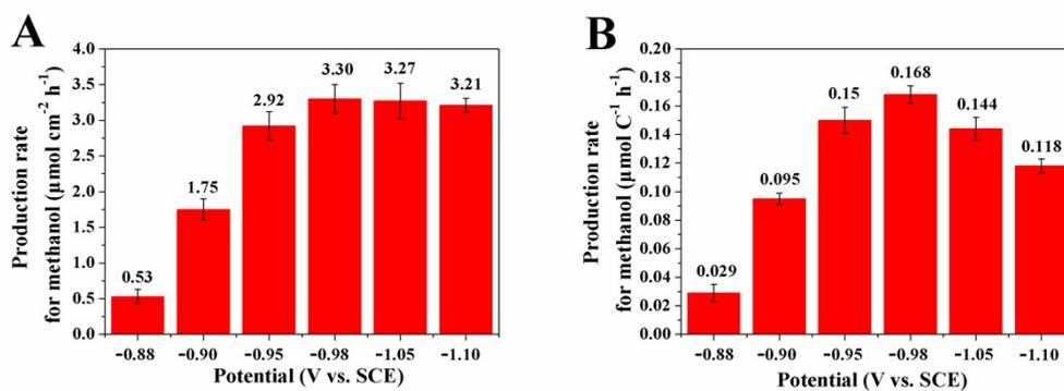
**Fig. S8** Production rates of methanol normalized by (A) available reaction area and (B) charge obtained from electrochemical reduction of  $\text{CO}_2$  for 10 h at hollow urchin-like  $\text{Co}(\text{CO}_3)_{0.5}(\text{OH}) \cdot 0.11\text{H}_2\text{O}$  under different applied electrolysis potentials.
