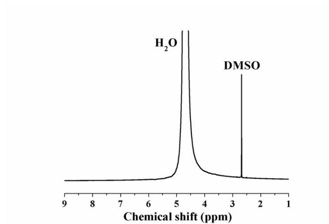
**Fig. S7** <sup>1</sup>H-NMR spectra of the electrolyte after electrolysis in N<sub>2</sub>-saturated 0.1 M NaHCO<sub>3</sub> aqueous solution at -0.98 V (vs. SCE) for 10 h at hollow urchin-like Co(CO<sub>3</sub>)<sub>0.5</sub>(OH)·0.11H<sub>2</sub>O.
