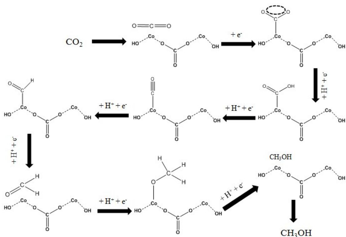
**Fig. S11** Possible high selectivity reaction mechanism for electrochemical reduction of CO<sub>2</sub> to CH<sub>3</sub>OH on hollow urchin-like Co(CO<sub>3</sub>)<sub>0.5</sub>(OH)·0.11H<sub>2</sub>O electrocatalyst in aqueous solution.
