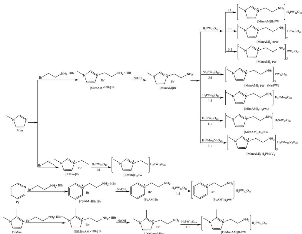
**Scheme S1** Synthesis of amino-functionalized HPA-based ionic hybrid catalysts and various counterparts
