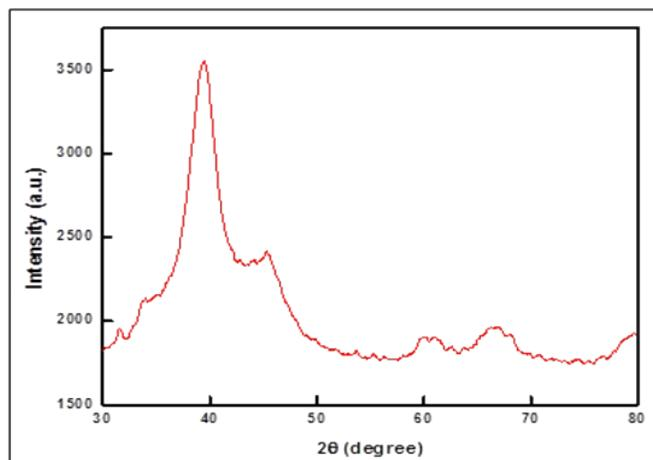
Fig. S5 XRD pattern of Pd-Ni NPs recovered after five catalytic cycles
