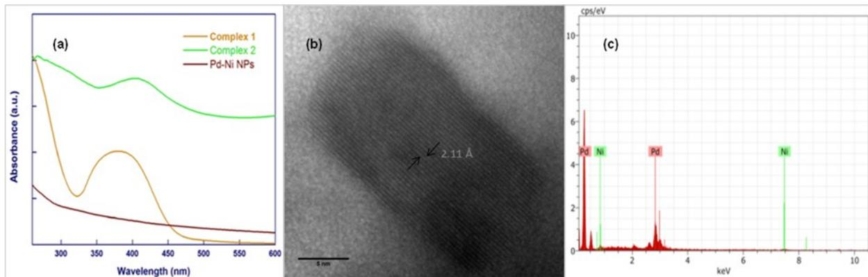
Fig. S2 (a) UV-Vis spectrum (b) HRTEM (c) EDS image of Pd-Ni NPs
