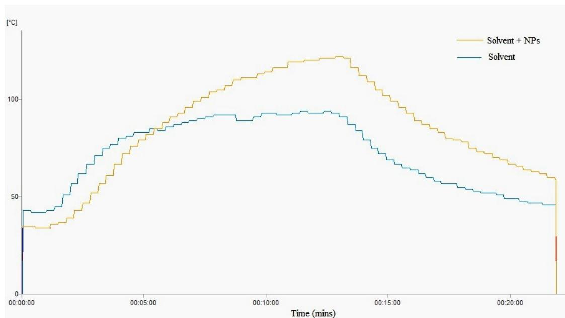
Fig. S4 Comparison of temperature profiles of system carrying blank solvent and solvent with NPs.
