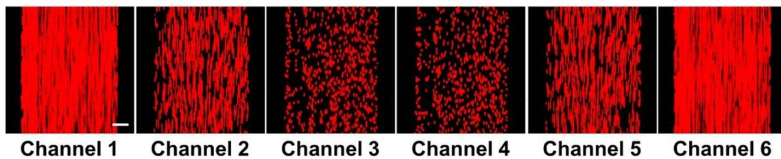
**Fig. S2** The fluorescent streak images of 7  $\mu\text{m}$  beads in six parallel channels with inlet velocity of 0.06 m/s. Scale bars: 100  $\mu\text{m}$ .
