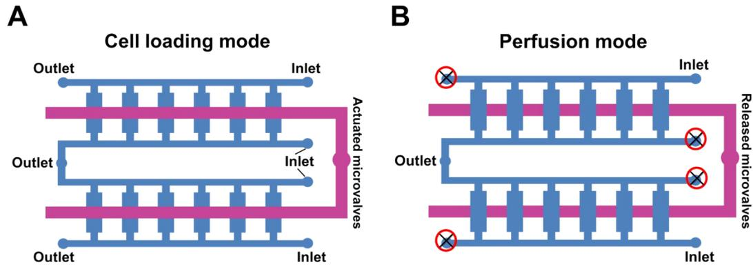
**Fig. S5** The schematic view of integrated microfluidic platform in two working mode.
