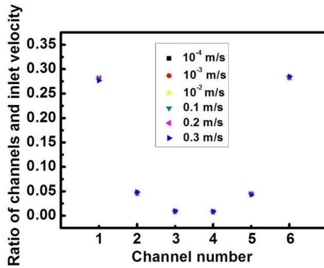
**Fig. S3** The simulation results of the distribution ratio of steady velocity in six parallel channels when inlet velocity ranged from  $10^{-4}$  m/s to 0.3 m/s.
