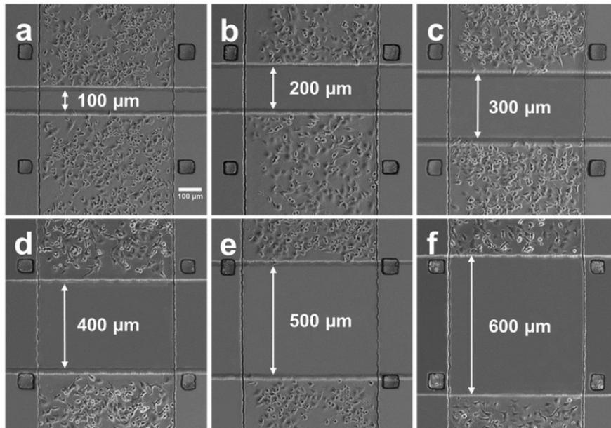
**Fig. S1** Different width regular exclusion zones could easily be realized by simply controlling width-variable microvalves on designed microfluidic platform. Scale bars: 100  $\mu\text{m}$ .
