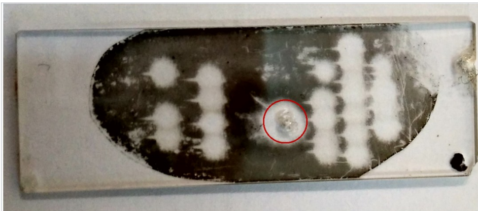
Figure S4. Photo of the rGO film on quartz substrate after its ablation during the experiments. As seen, no fragmentation of substrate can be observed in multiple areas of GO film ablation. The marked spot indicates area where substrate was advisedly disrupted after 15 consecutive laser pulses.
