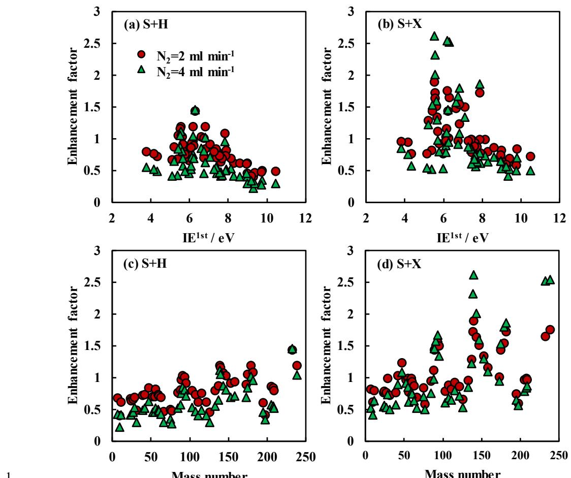
1 SFig.1 Correlation of IE<sup>1st</sup> and mass number and signal enhancement factor for nitrogen addition (N<sub>2</sub>= 2 and 4 ml min<sup>-1</sup>) in S+H (a and c) and S+X (b and d) cone.
