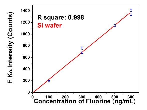
**Figure S1:** Calibration plot obtained for the TXRF determination of F in water samples with F concentration in the range of 100-600 ng/mL. The samples were deposited on Si wafer supports
