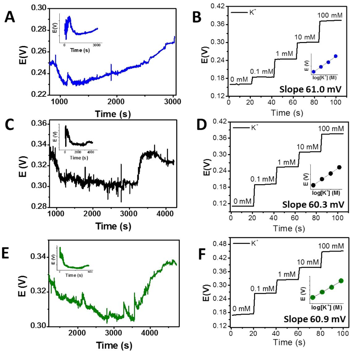
Figure S2. A, C, E) Monitoring of sweat potassium during cycling exercise from three health volunteers. Insets show on-body results starting from time 0 seconds. B, D, F) Calibration curves of potassium sensor before these on-body tests. Insets show  $E$  vs  $\log [K^+]$  (mM) plot along with the slope for each calibration.
