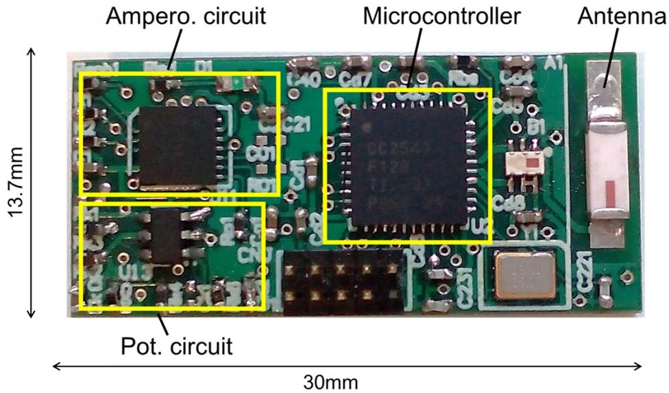
Figure S7. Amperometric and potentiometric PCB board.
