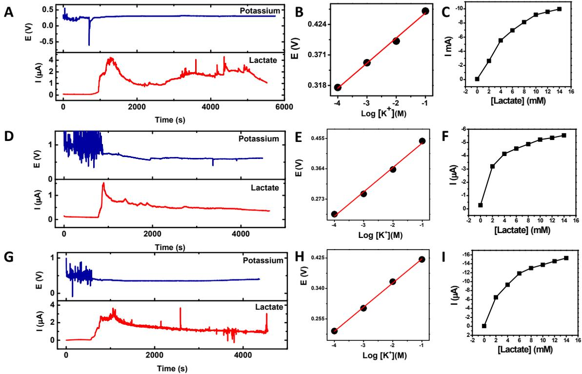
Figure S4. A, D, G) Simultaneous sweat potassium and lactate monitoring during cycling exercise from three volunteers. B, E, H) Potassium calibration plots obtained before on-body tests. C, F, I) lactate calibration curves before on-body tests.
