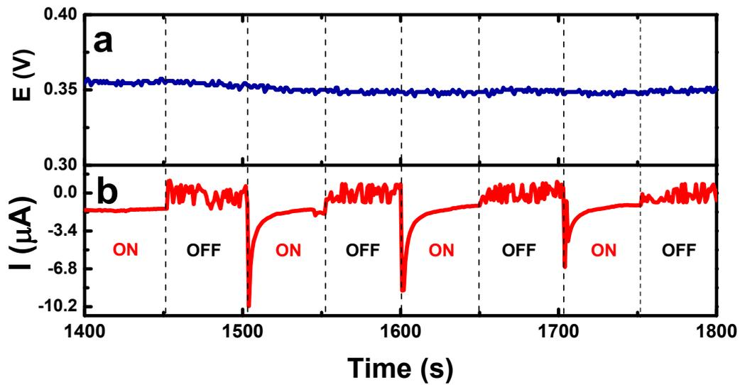
Figure S5. Cross-talk experiment between the potassium (a) and lactate (b) sensors during on-body test using wireless MAG device.
