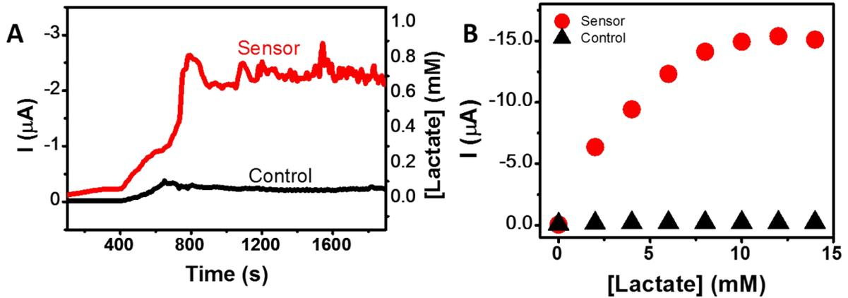
Figure S3. A) Monitoring of sweat lactate during cycling exercise. B) Calibration curves for the lactate biosensor and enzyme-free control sensor before on-body tests.
