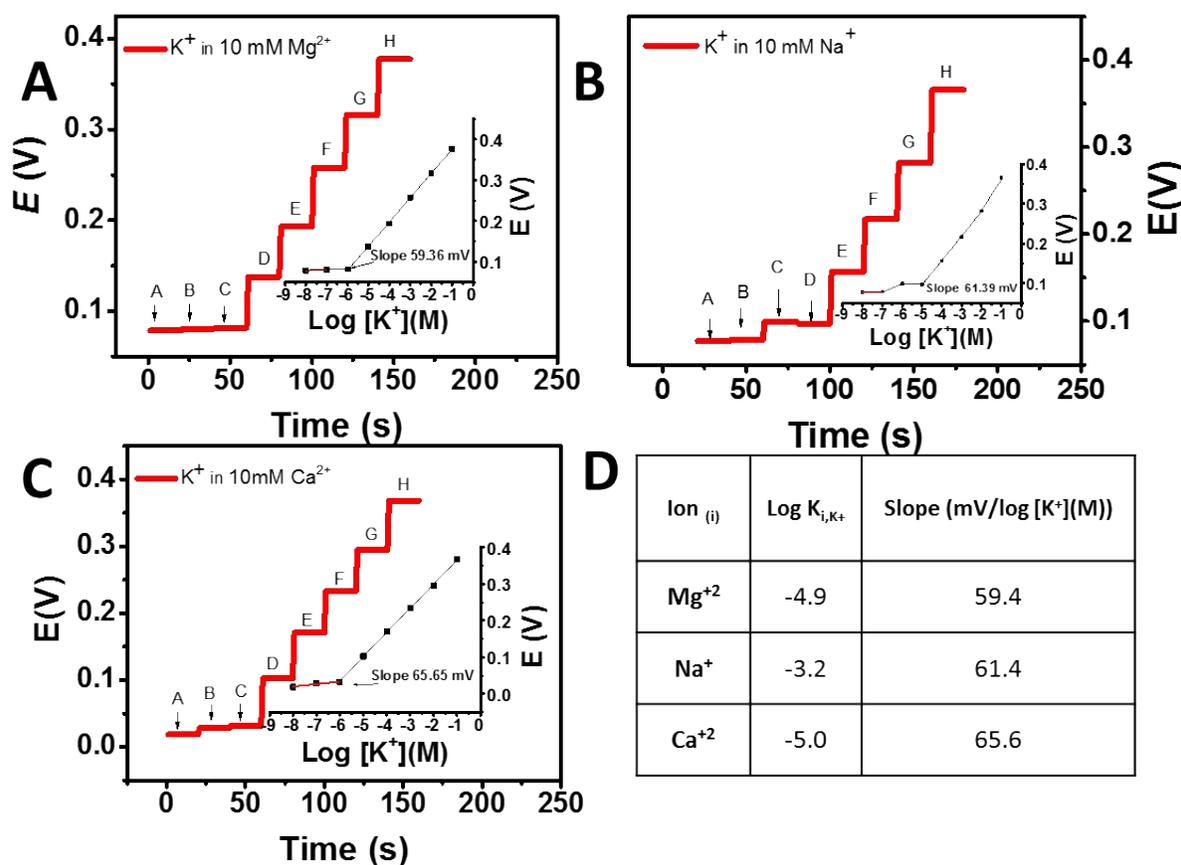
Figure S1. Selectivity coefficient determination using the fixed solution method. Response of  $1 \times 10^{-5}$  –  $1 \times 10^2$  mM (A-H) potassium concentrations and respective calibration curves (insets) in 10 mM of A) Magnesium, B) Sodium and C) Calcium. D) Table with selective coefficient and slope for potassium response in 10 mM of magnesium, sodium, and calcium respectively.
