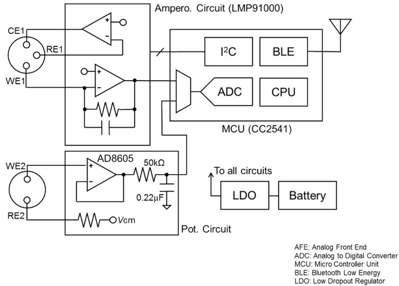
Figure S6. Block diagram of glasses sensor circuit board.
