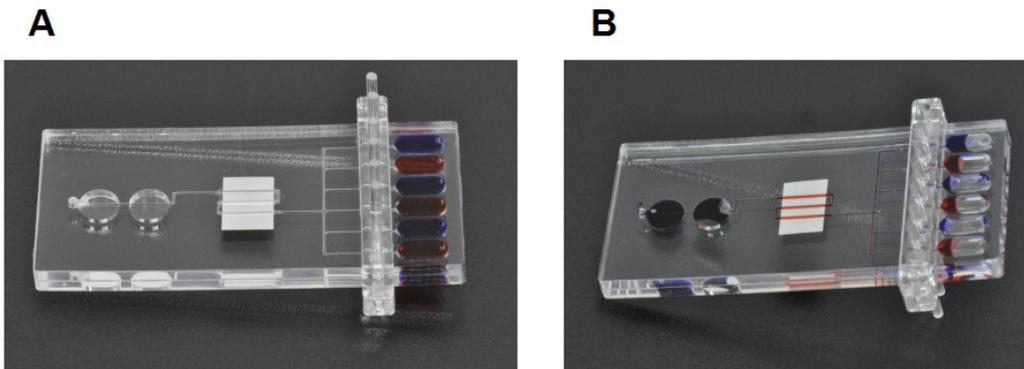
**Fig. S3** The photographs of microfluidic chip before (A) and after (B) automated immunoassay. In order to improve visual effect, two different colored dyes are loaded into the inlet reservoirs.
