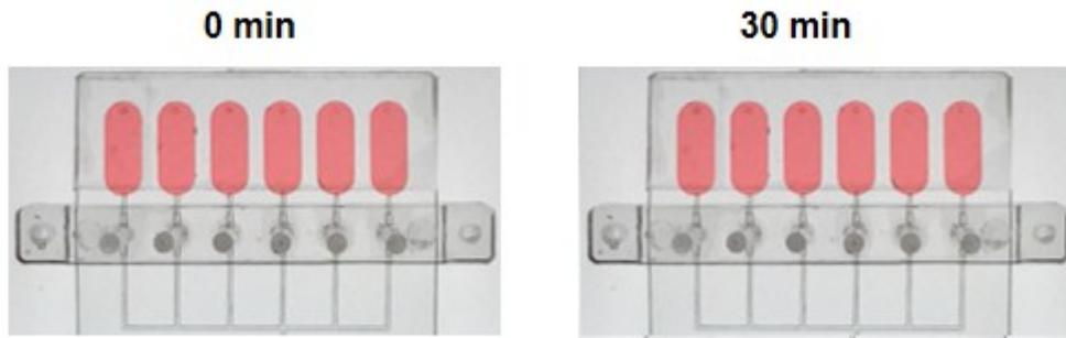
**Fig. S2** Baking experiment to test sealing effect of on-chip valves at initial closed state. The baking experiment contains three steps: (1) injecting the red-colored liquid into the six inlet reservoirs; (2) sealing the air holes on reservoirs by 3M adhesive tape; (3) baking the microfluidic device inside an oven at 85 °C for 30 min. No leakage of liquid into the downstream microchannels is observed before and after baking.
