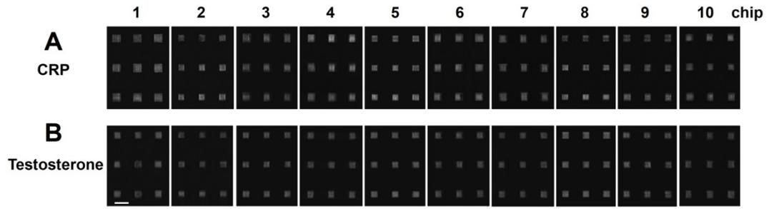
**Fig. S4** Reproducibility test. (A) Images of ten chips for CRP (200 ng/mL) detection. (B) Images of ten chips for testosterone (10 ng/mL) detection. Scale bar is 1000  $\mu\text{m}$ .
