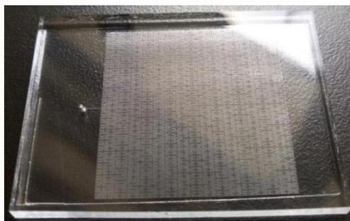
**Figure S3.** Photograph of the high-density self-priming fractal branching microfluidic nets digital PCR chip. The chip has 14 branching levels only in one fractal dimension which contains 16384 microchambers. The volume of the reaction chamber is  $150\ \mu\text{m} \times 150\ \mu\text{m} \times 250\ \mu\text{m}$ , the size of the circulation channel is  $50\ \mu\text{m} \times 25\ \mu\text{m}$ . The chip size is  $40\ \text{mm} \times 60\ \text{mm}$ .
