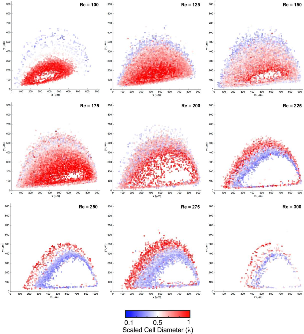
**Supplementary Figure 3. Scatter plot of captured cells size distribution and their orbit trajectories in AR = 1 cavity.** Cell motion and progression in microvortices illustrates size selective orbit transition in increasing flow conditions at Reynolds number (Re) 100, 125, 150, 175, 200, 225, 250, 275 and 300.
