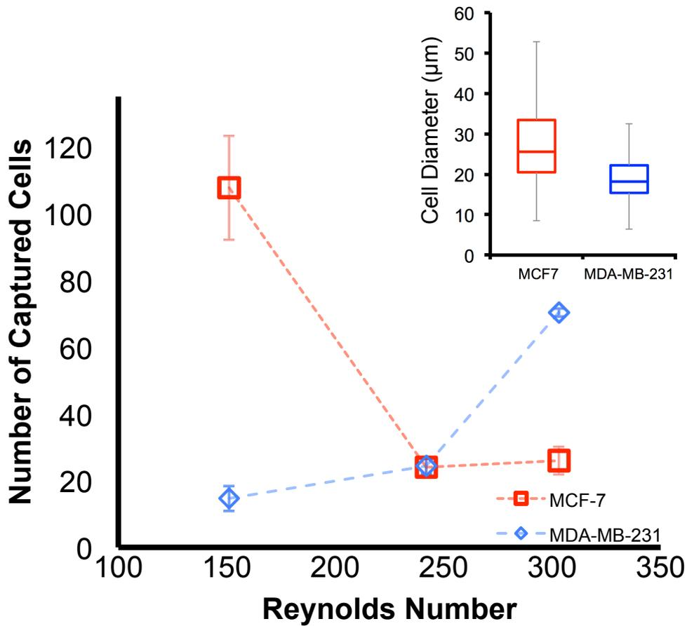
**Supplementary Figure 4. Microvortex loading capacity of MCF-7 ( $\lambda > 0.5$ ) cells) and MDA-MB-231 ( $\lambda < 0.5$ ).** Flow of concentrated cell suspension for five minutes followed by PBS wash for five minutes in three inertial conditions at  $Re = 150, 240$  and  $300$ . Microvortex capture of MCF-7 with mean cell diameter =  $25 \mu\text{m}$  and MDA-MB-231 =  $18 \mu\text{m}$  show size-selective capacity in phase I ( $Re = 150$ ) and phase III ( $Re = 275$ ) respectively.
