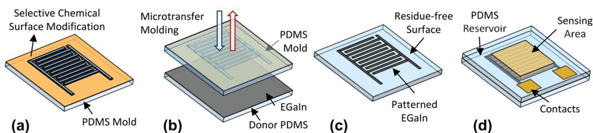
**Fig. S1** An advanced EGaln patterning process for scalable, uniform, and residue-free EGaln thin-line fabrication: (a) selective chemical surface modification of the PDMS mold, (b) microtransfer molding of EGaln, (c) EGaln-filled PDMS mold after residue transfer, and (d) microfluidic integration and vertical interconnection.<sup>29,30</sup>
