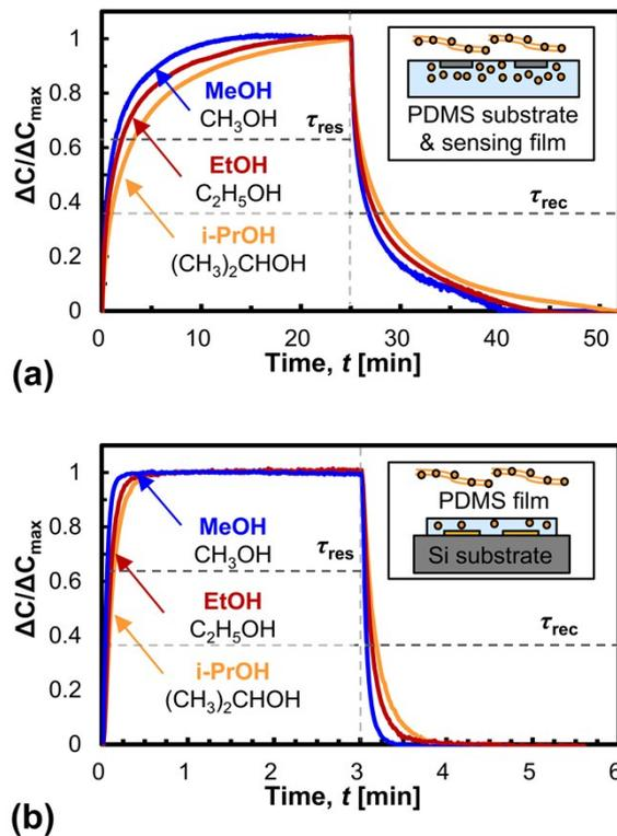
**Fig. S4** Transient signal responses, i.e. normalized capacitance changes, during analyte absorption and subsequent analyte desorption for (a) all-soft sensor (b) solid-state sensor with a PDMS sensing film upon exposure to isopropanol (i-PrOH), ethanol (EtOH), and methanol (MeOH).
