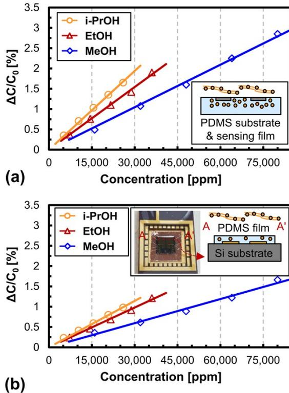
**Fig. S3** Measured relative capacitance changes of (a) all-soft sensor and (b) solid-state sensor with a PDMS sensing film as a function of the analyte concentrations of isopropanol (i-PrOH), ethanol (EtOH), and methanol (MeOH).
