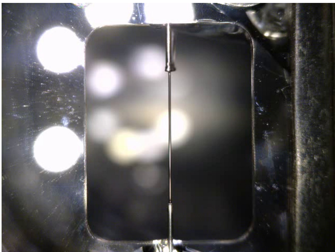
Fig. A1 The PMMA frame is micromachined to accommodate both the fiber probe and the capillary for the jet ejection on the same axis. The stable flow rate and the PMMA frame guarantee a self-alignment condition.
