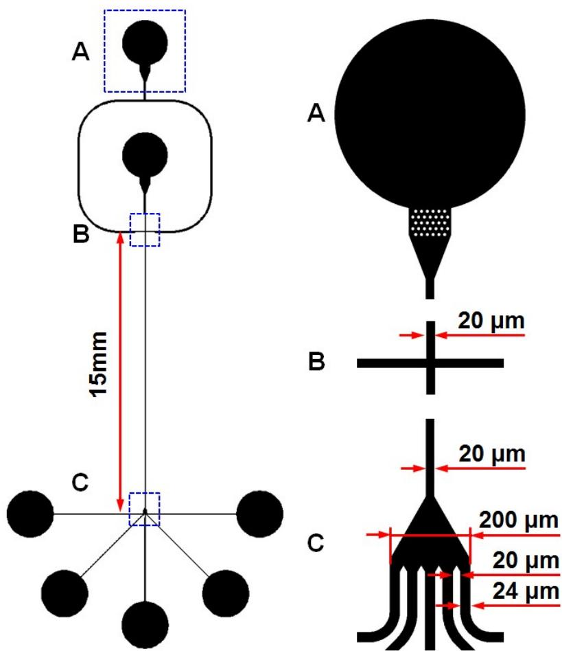
**Figure S1.** The microchannel design. The microfluidic device consists of two identical inlets with debris filters for sheath and sample flows, a separation channel (15 mm long and 20  $\mu\text{m}$  wide), and five outlets for small particles (two side outlets) and large particles (three center outlets). The width of all the outlets is 24  $\mu\text{m}$ . The entire microchannel has a uniform height of 50  $\mu\text{m}$ .
