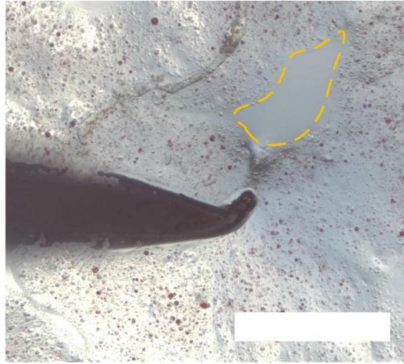
**Figure S6:** Detail of the container's surface after 6 s of spraying at 11 cm distance. The right image shows a needle deforming the container. A dashed line is used to highlight a spot that is not covered by the DS10 coating. Scale bar 400  $\mu\text{m}$ .
