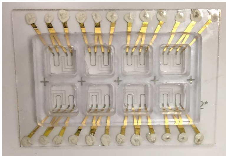
Figure S17 | 8-Well device prototype applied in initial tests and NRVM-based experiments.
