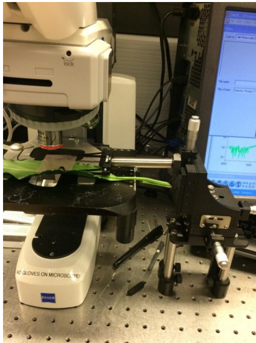
Figure S2. A set for microfluidic leaf printing (left – disassembled and right – assembled): a microfluidic chip placed between leaf veins and two plastic holders for clamping. The top holder has an opening to insert ink into the microfluidic chip after clamping. Red arrow points on microfluidic chip. (Bottom) Microfluidic chip is aligned on top leaf surface using XYZ translational stage.
