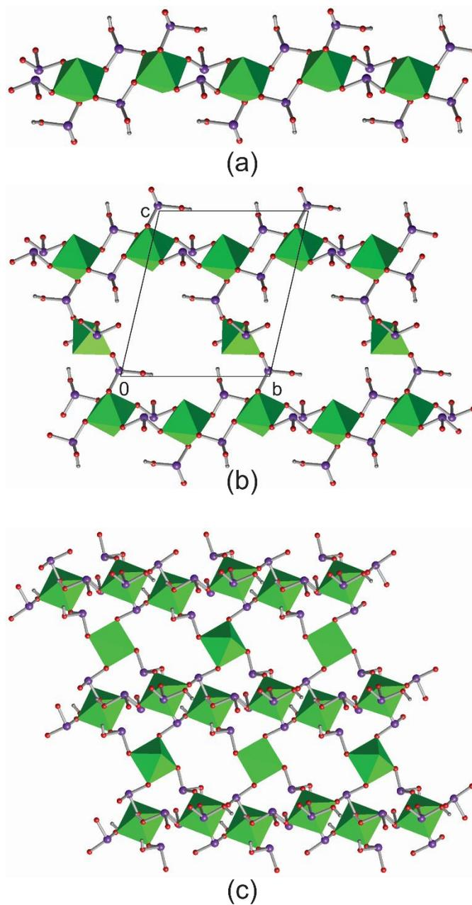
**Figure S3.** (a) One-dimensional chain SBU and (b) and (c) two slice connectivities in  $[\text{C}_4\text{H}_{12}\text{N}_2][(\text{VO})_3(\text{SeO}_3)(\text{HSeO}_3)_4]\cdot\text{H}_2\text{O}$  (4). Green polyhedra represent  $[\text{VO}_6]$  and  $[\text{VO}_5]$  while purple, red, and gray spheres represent selenium oxygen, and hydrogen atoms, respectively.
