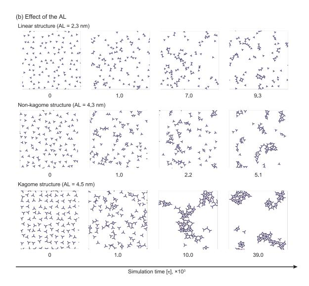
Fig. S1 Representative snapshots of self-assembly process for the whole simulation box. (a) As for the effect of HR, three characteristic phases, a non-ordered phase, a kagome structure phase, and a non-kagome structure phase, were observed in the nanoslit. (b) As for the effect of AL, three characteristic phases including a linear-structure phase, a non-kagome structure phase, and the kagome structure phase, depending on the value of AL.
