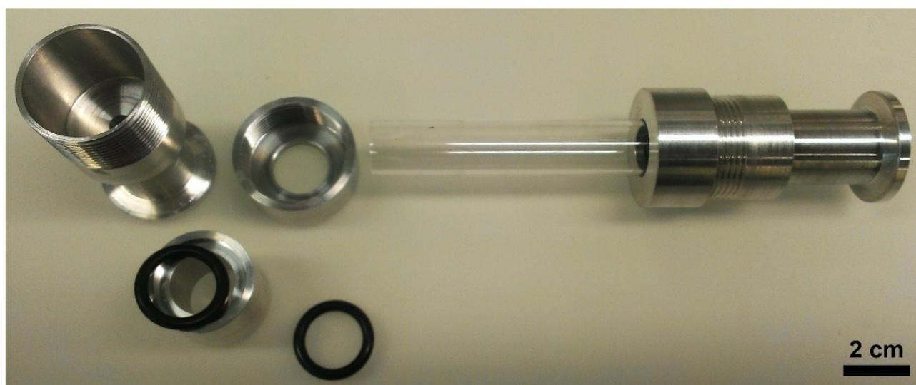
**Figure S1** Photograph of the different reactor components with half of the setup assembled.
