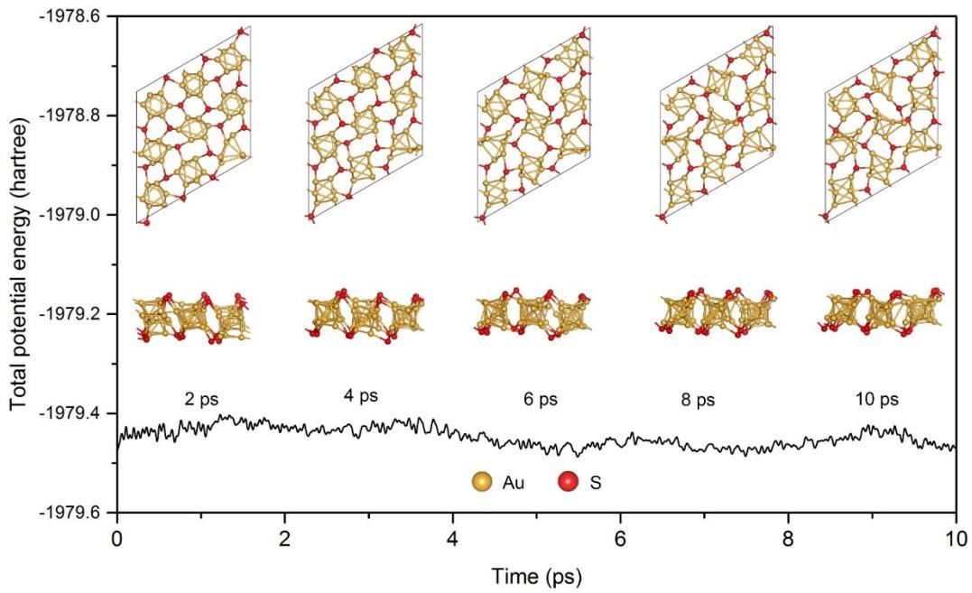
**Figure S7.** *Ab initio* MD results for T-Au<sub>6</sub>S<sub>2</sub> monolayer. Total potential energy as function of MD time were plotted. Snapshot at 2 ps, 4 ps, 6 ps, 8 ps and 10 ps are inserted inside.
