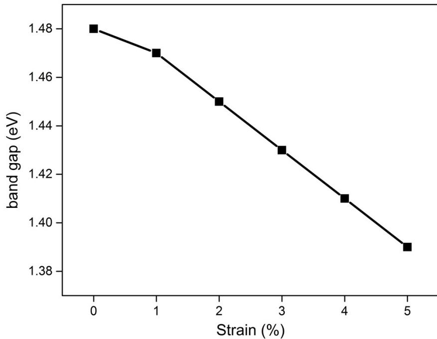
**Figure S9.** Strain effect on the band gap of T-Au<sub>6</sub>S<sub>2</sub> monolayer.
