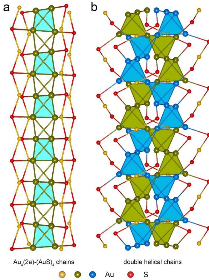
**Figure S3.** (a)  $\text{Au}_4(2e)$ - $(\text{AuS})_4$  chain in G- $\text{Au}_6\text{S}_2$  monolayer. (b) Double helical chains composed of tetrahedral  $\text{Au}_4(2e)$  elementary blocks are protected by staple motifs [Taken from the reference “Xu, W. W.; Li, Y.; Gao, Y.; Zeng, X. C. Unraveling a generic growth pattern in structure evolution of thiolate-protected gold nanoclusters. *Nanoscale*, **2016**, *8*, 7396–7401”].
