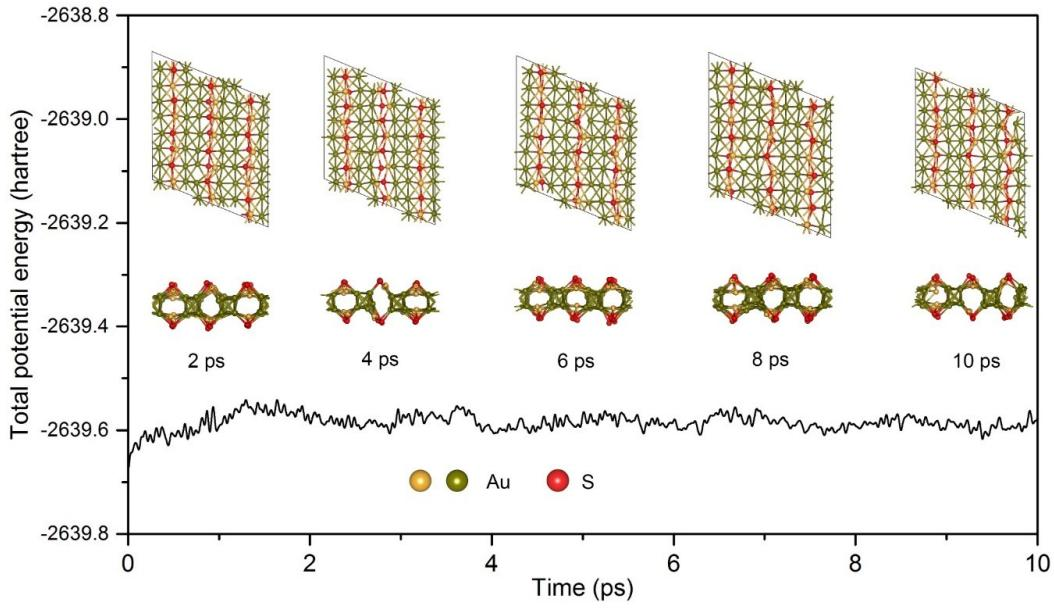
**Figure S6.** *Ab initio* MD results for G-Au<sub>6</sub>S<sub>2</sub> monolayer. Total potential energy as function of MD time were plotted. Snapshot at 2 ps, 4 ps, 6 ps, 8 ps and 10 ps are inserted inside.
