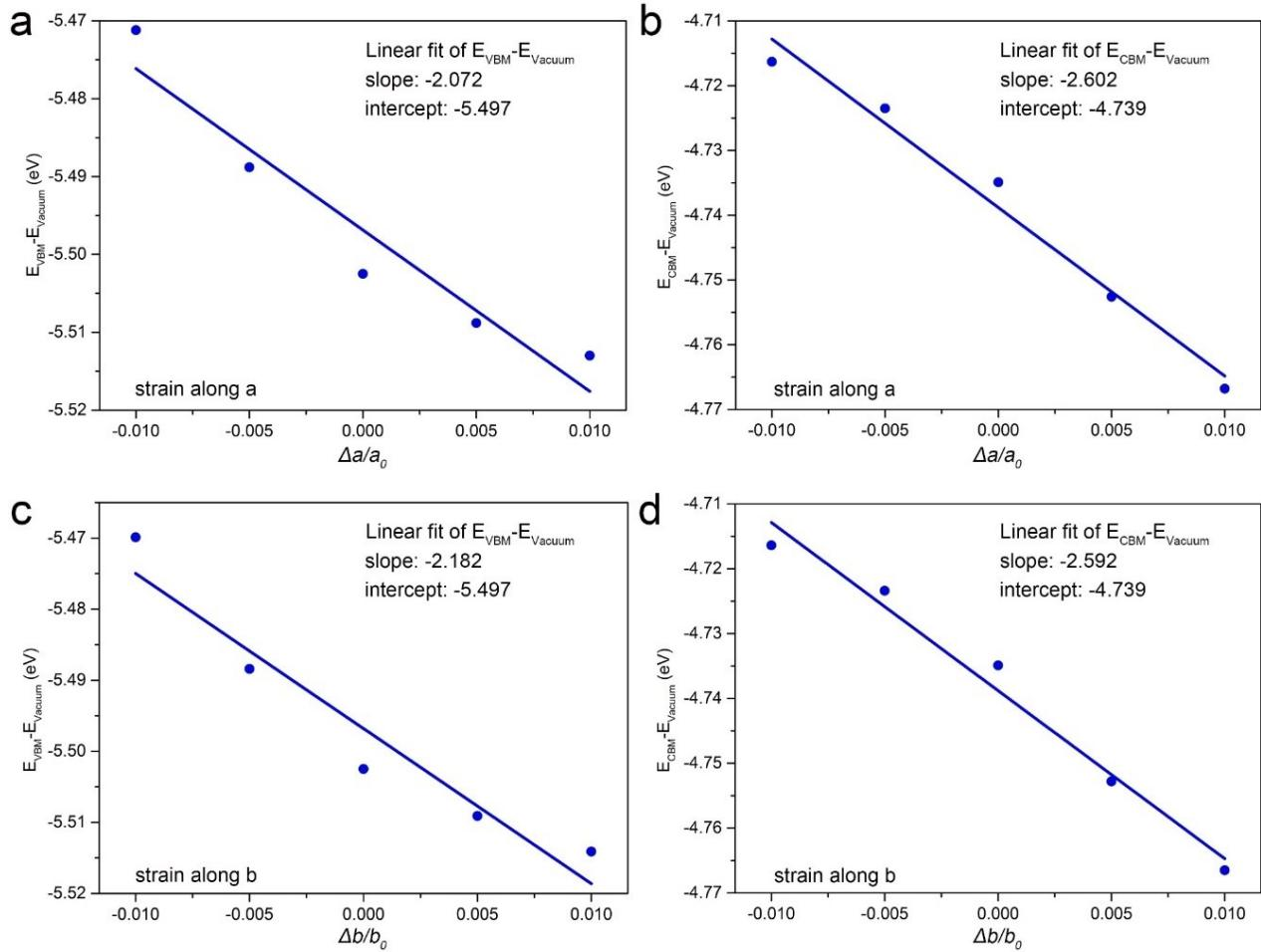
**Figure S12.** Linear fitting of deformation potential. Band energy of the VBM (a, c) and CBMs (b, d) of  $\text{Au}_6\text{S}_2$  monolayer with respect to the vacuum energy as a function of lattice dilation. PBE-GGA functional with SOC considered was adopted to compute deformation potential constant for reducing the huge computational cost.
