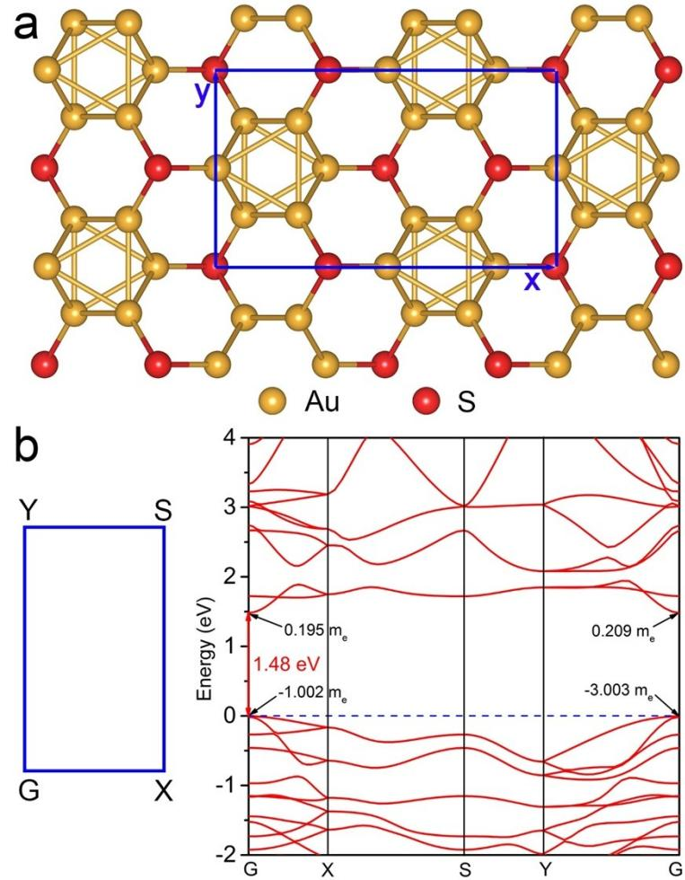
**Figure S11.** (a) Representative structure of rectangle cell of T-Au<sub>6</sub>S<sub>2</sub> monolayer as indicated with blue lines and texts. (b) Sketch for Brillouin zone and band structures calculated based on HSE06 functional. Band gap and effective electron/hole masses are noted inside.
