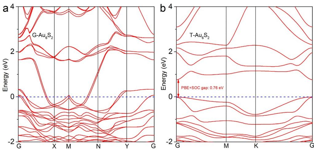
**Figure S8.** Computed band structures of G-Au<sub>6</sub>S<sub>2</sub> (a) and T-Au<sub>6</sub>S<sub>2</sub> (b) at PBE level. Spin-orbit coupling (SOC) was considered.
