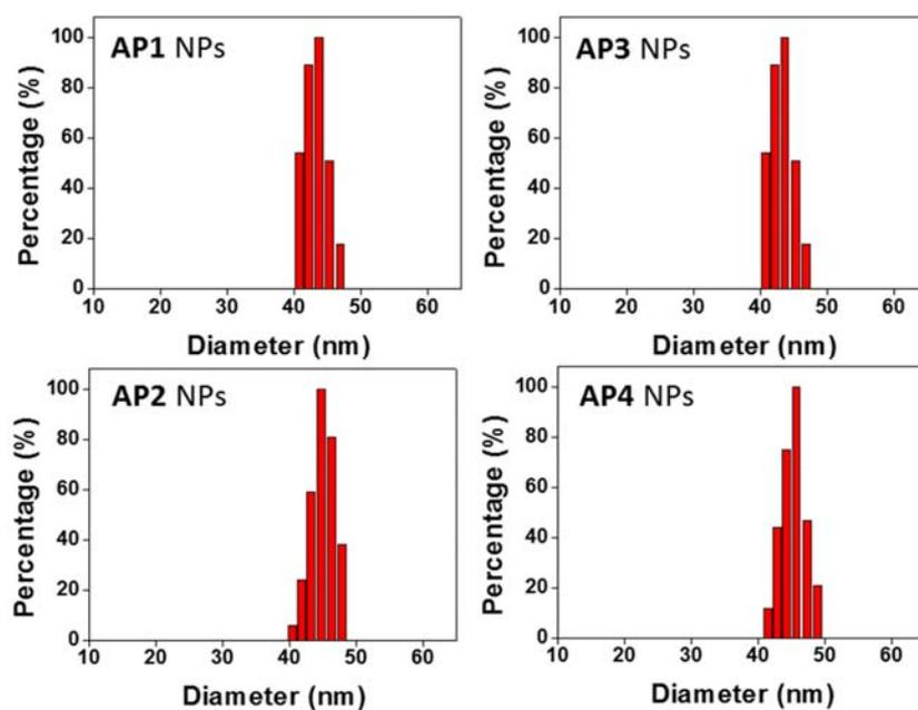
**Fig. S13.** Dynamic laser scattering (DLS) results of AP1-AP4 NPs.
