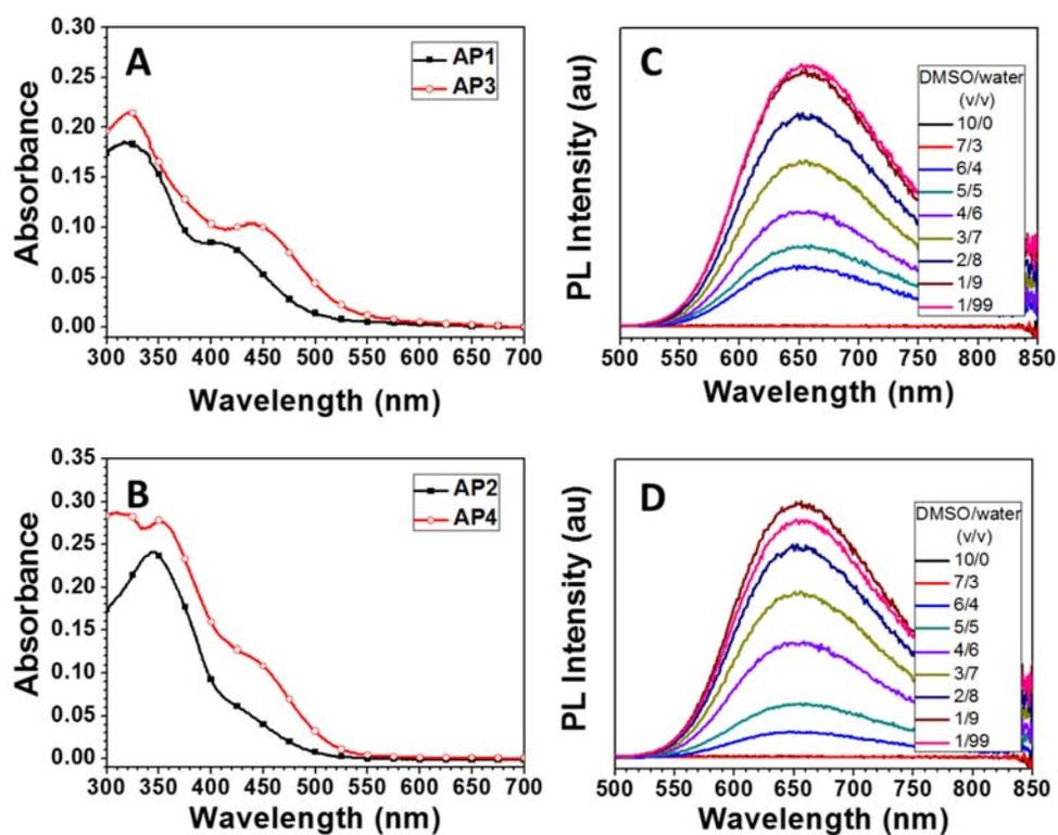
**Fig. S8.** (A, B) UV-vis spectra of AP1, AP3 (A) and AP2, AP4 (B) in DMSO/water = 1/99 (v/v). (C, D) PL spectra of AP3 (C) and AP4 (D) in DMSO and DMSO-water mixtures at different volume ratios ( $\lambda_{\text{ex}} = 460 \text{ nm}$ ). [AP1 or AP2 or AP3 or AP4] =  $5 \times 10^{-6} \text{ M}$ .
