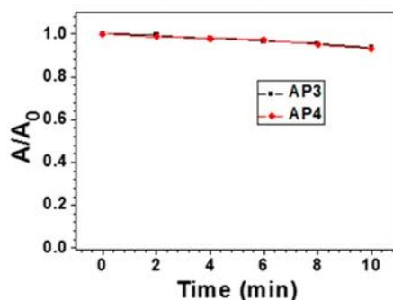
**Fig. S9.** The degradation rates of AP3 and AP4 under light irradiation ( $60 \text{ mW/cm}^2$ , 400-700 nm).  $A_0$  and  $A$  are the absorbance of AP3 or AP4 at 450 nm before and after light irradiation, respectively. [AP3 or AP4] =  $10 \text{ }\mu\text{g/mL}$ .
