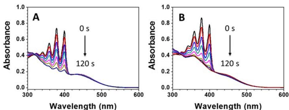
**Fig. S15.** UV-vis spectra of ABDA in the presence of AP3 NPs (A) or AP4 NPs (B) under light irradiation ( $60 \text{ mW/cm}^2$ , 400-700 nm) in water. [AP3 or AP4 NPs] =  $10 \text{ }\mu\text{g/mL}$  based on AP3 or AP4 molecule, [ABDA] =  $5 \times 10^{-5} \text{ M}$ .
