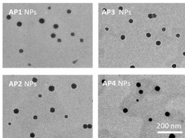
**Fig. S12.** Transmission electron microscopy (TEM) images of AP1-AP4 NPs. All the TEM images share the same scale bar of 200 nm.
