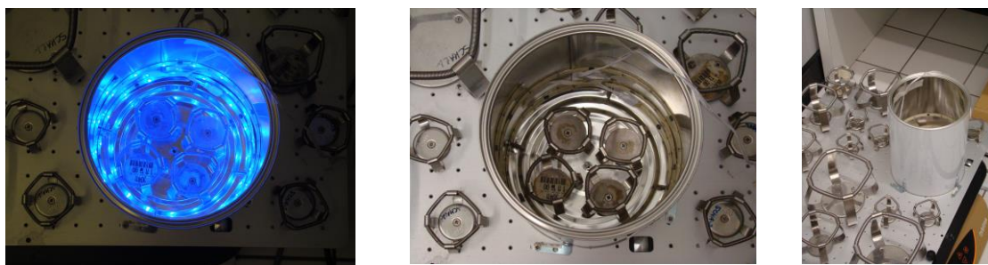
Fig. S27. Pictures of the irradiation device. 45 LEDs (3.45 W, 25 Lumen, FlexLED Inspire; www.erp-inspire.com ) arranged helicoidally inside a metal cyclinder ( h = 22 cm, diam.= 18 cm). A video is available on https://youtu.be/gMmTJuYzAhY .
