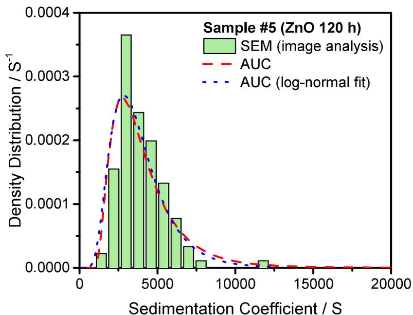
**Figure S5** Analysis results for ZnO NR sample #5. Expected sedimentation coefficient distribution obtained from theoretical calculations from SEM image analysis, normalized distributions obtained from AUC measurements and the log-normal distribution fit to the AUC data.
