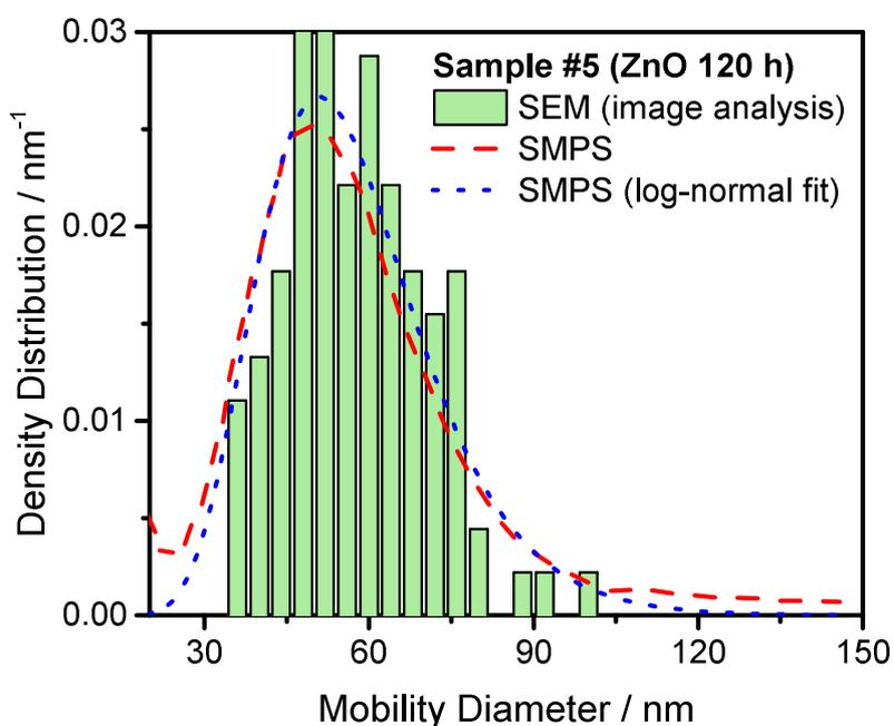
**Figure S6** Analysis results for ZnO NR sample #5. Expected mobility diameter distribution obtained based on theoretical calculations from SEM image analysis, normalized distributions obtained from SMPS measurements and the log-normal distribution fit to the SMPS data.
