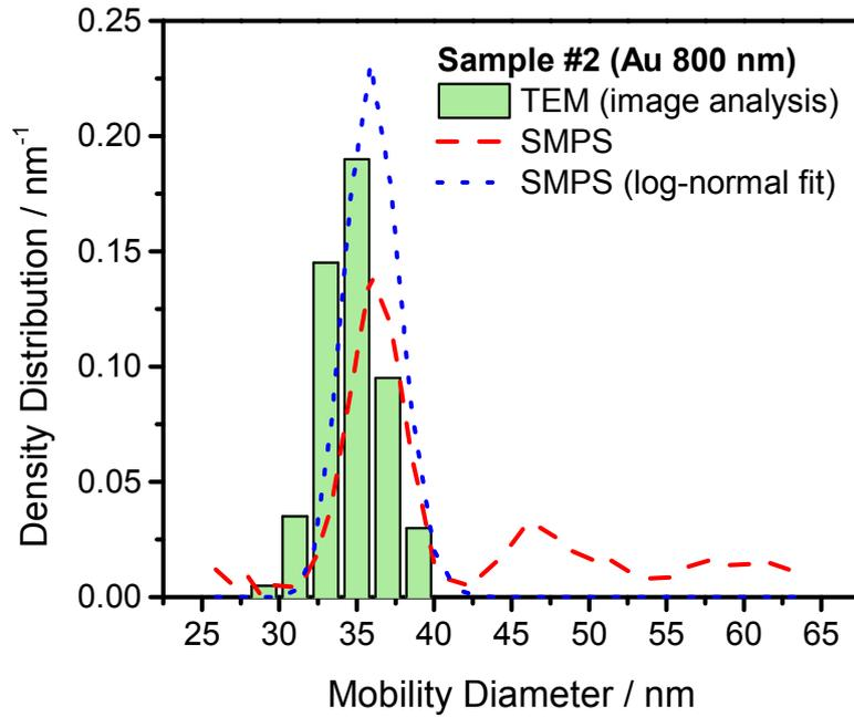
**Figure S2** Analysis results for Au NR sample #2. Expected mobility diameter distribution obtained based on theoretical calculations from TEM image analysis, normalized distributions obtained from SMPS measurements and the log-normal distribution fit to the SMPS data.
