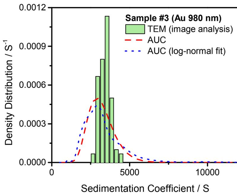
**Figure S3** Analysis results for Au NR sample #3. Expected sedimentation coefficient distribution obtained from theoretical calculations from TEM image analysis, normalized distributions obtained from AUC measurements and the log-normal distribution fit to the AUC data.
