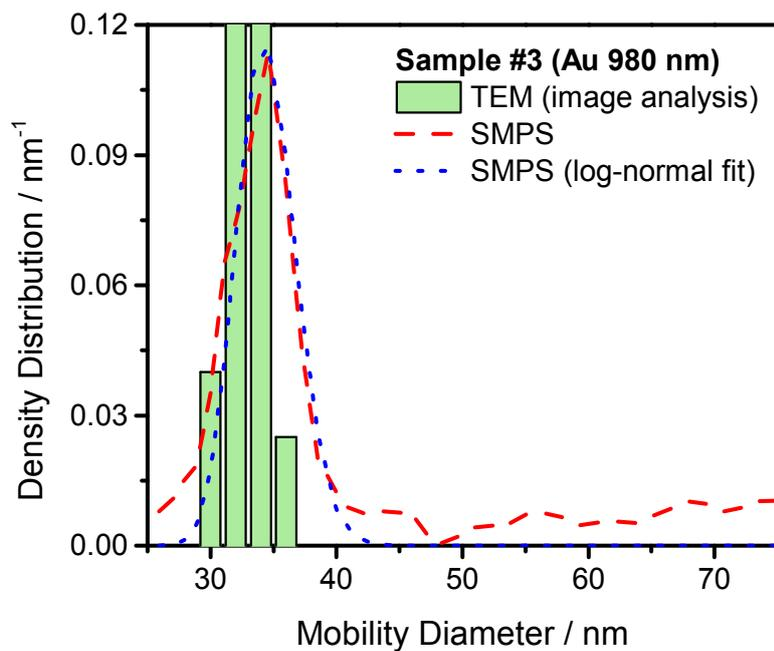
**Figure S4** Analysis results for Au NR sample #3. Expected mobility diameter distribution obtained based on theoretical calculations from TEM image analysis, normalized distributions obtained from SMPS measurements and the log-normal distribution fit to the SMPS data.
