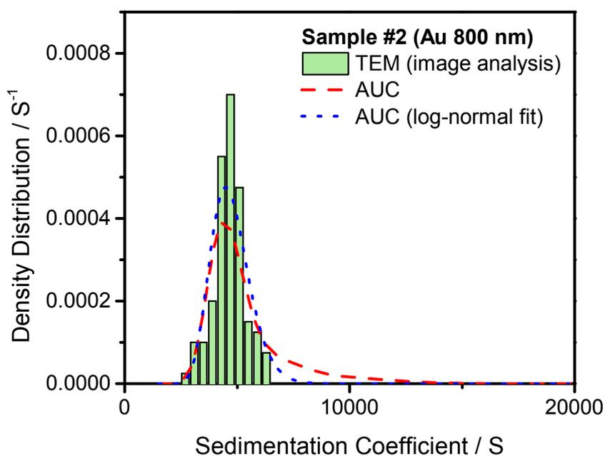
**Figure S1** Analysis results for Au NR sample #2. Expected sedimentation coefficient distribution obtained from theoretical calculations from TEM image analysis, normalized distributions obtained from AUC measurements and the log-normal distribution fit to the AUC data.
