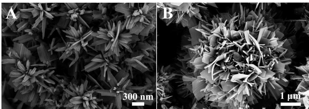
**Fig. S2** FESEM images of  $\text{NiCo}_2\text{S}_4$  without template.
