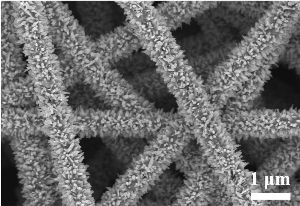
**Fig. S1** FESEM images of NiCo<sub>2</sub>S<sub>4</sub>@CNF hybrid.
