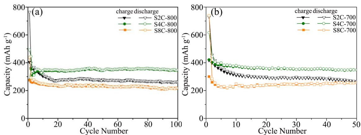
**Fig. S5.** Cycling performance at 100 mA g<sup>-1</sup> for S2C-800, S4C-800, S8C-800 (a), and S2C-700, S4C-700, S8C-700 (b).
