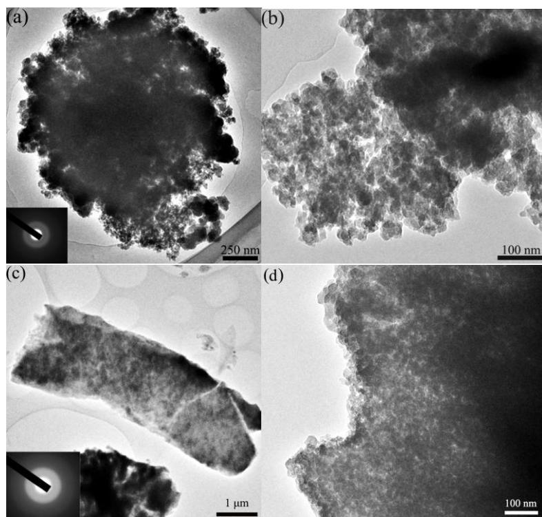
**Fig. S3.** HRTEM images of S2C-600 (a, b), S8C-600 (c, d). The insets are the corresponding EDP.
