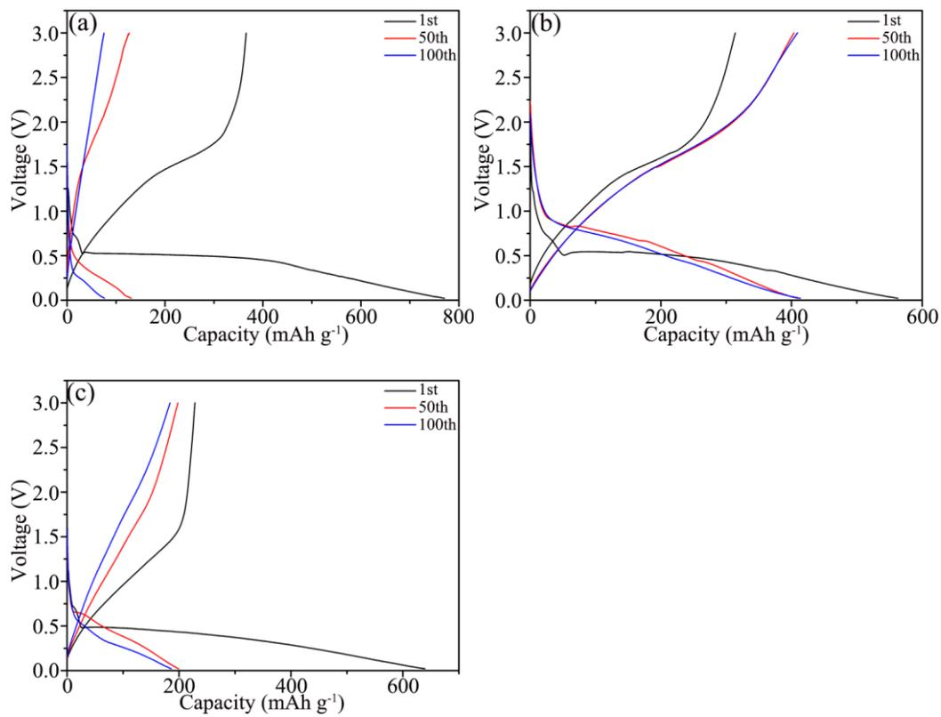
**Fig. S6.** Charge–discharge curves at 100 mA g<sup>-1</sup> for S2C-600 (a), S4C-600 (b), S8C-600 (c).
