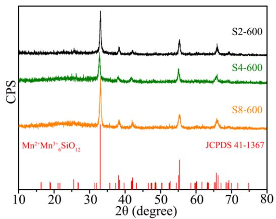
**Fig. S2.** XRD patterns of the products obtained by water-boiling treatment and subsequently heating at 600 °C in N<sub>2</sub> atmosphere.
