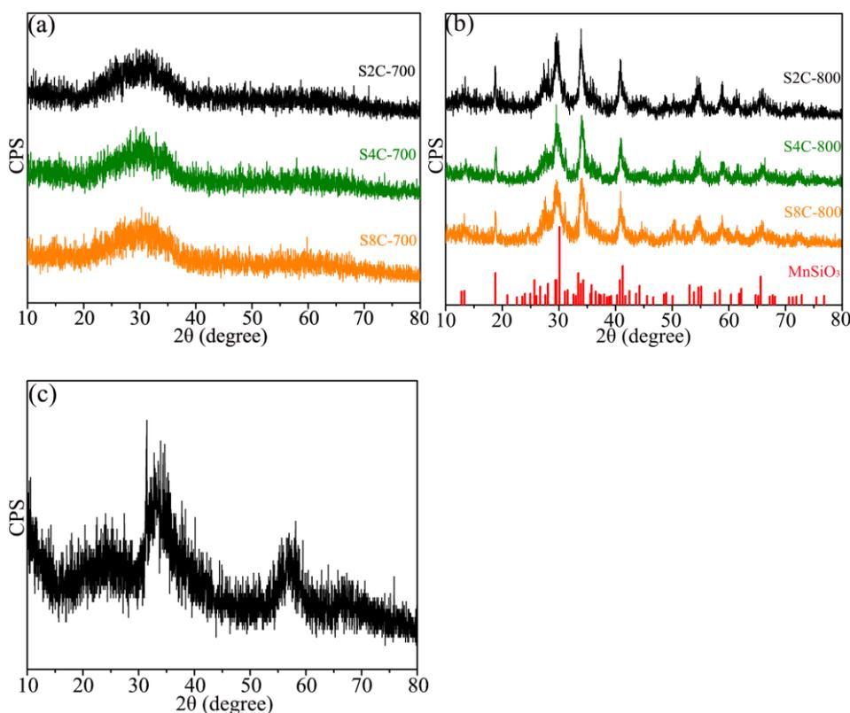
**Fig. S1.** XRD patterns of the carbon-coated products obtained at 700 °C (a), 800 °C (b), the product obtained by hydrothermally treating the mixed solution of  $\text{Na}_2\text{SiO}_3 \cdot 9\text{H}_2\text{O}$  and  $\text{MnCl}_2 \cdot 4\text{H}_2\text{O}$  at 180 °C for 8h (c).
