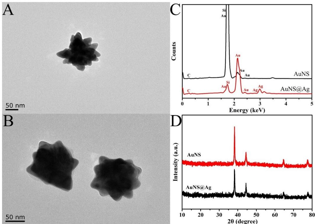
Figure S1. TEM images of (A) AuNS and (B) AuNS@Ag. (C) EDS spectra of AuNS@Ag and AuNS. (D) XRD patterns of AuNS@Ag and AuNS.
