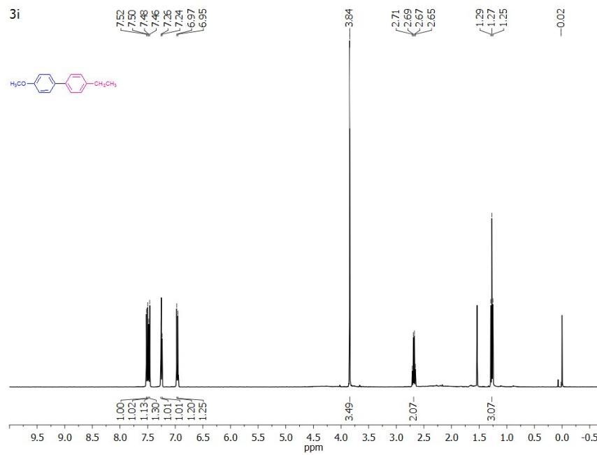
**Fig. S16:**  $^1\text{H}$  NMR of 4-methoxy-4-ethyl biphenyl (3i)
