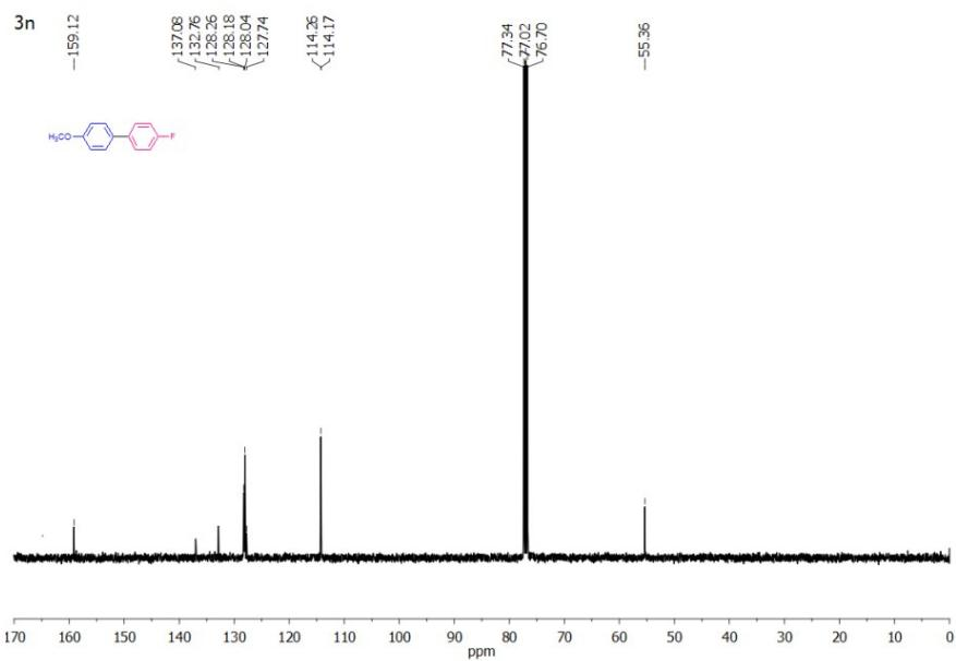
**Fig. S24:**  $^{13}\text{C}$  NMR of 4-methoxy-4-fluorobiphenyl (3n)
