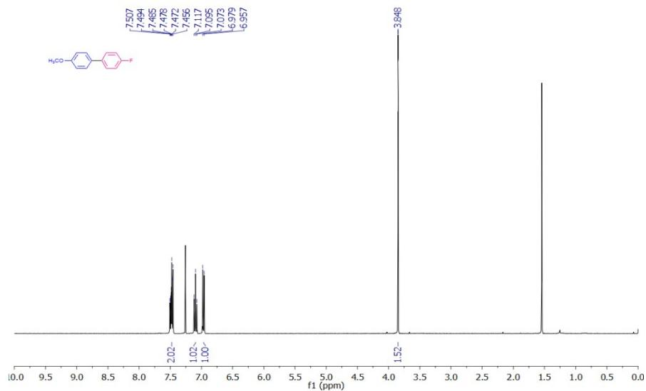
**Fig. S23:**  $^1\text{H}$  NMR of 4-methoxy-4-fluoro biphenyl (3n)
