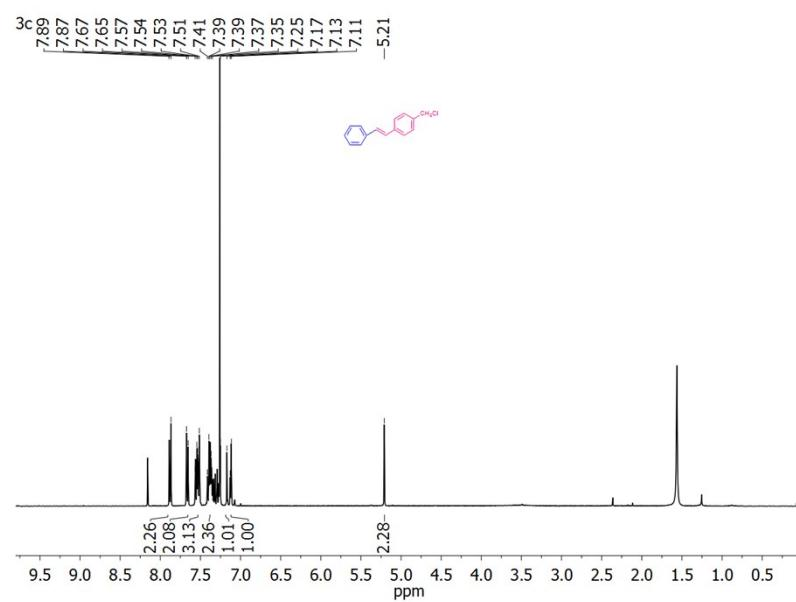
**Fig. S31:**  $^1\text{H}$  NMR of 4-chloromethylene trans-stilbene (3c)
