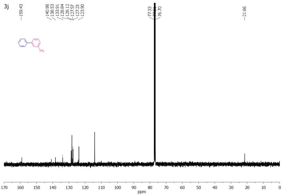
**Fig. S18:**  $^{13}\text{C}$  NMR of 3-methyl biphenyl (3j)
