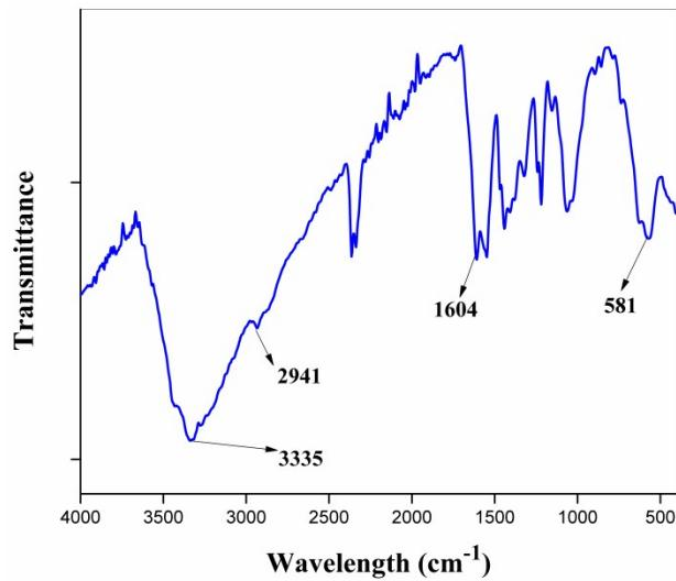
**Fig. S3.** FT-IR of reusable  $\text{Fe}_3\text{O}_4@\text{CS-SB-Pd}$  nanocatalyst after 5<sup>th</sup> cycle.
