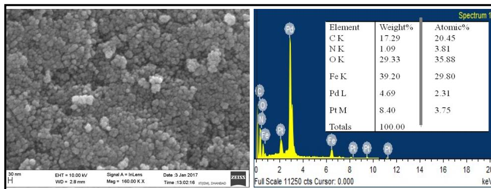
**Fig. S4.** FESEM image and EDX analysis of  $\text{Fe}_3\text{O}_4@\text{CS-SB-Pd}$  nanocatalyst after 5<sup>th</sup> cycle.
