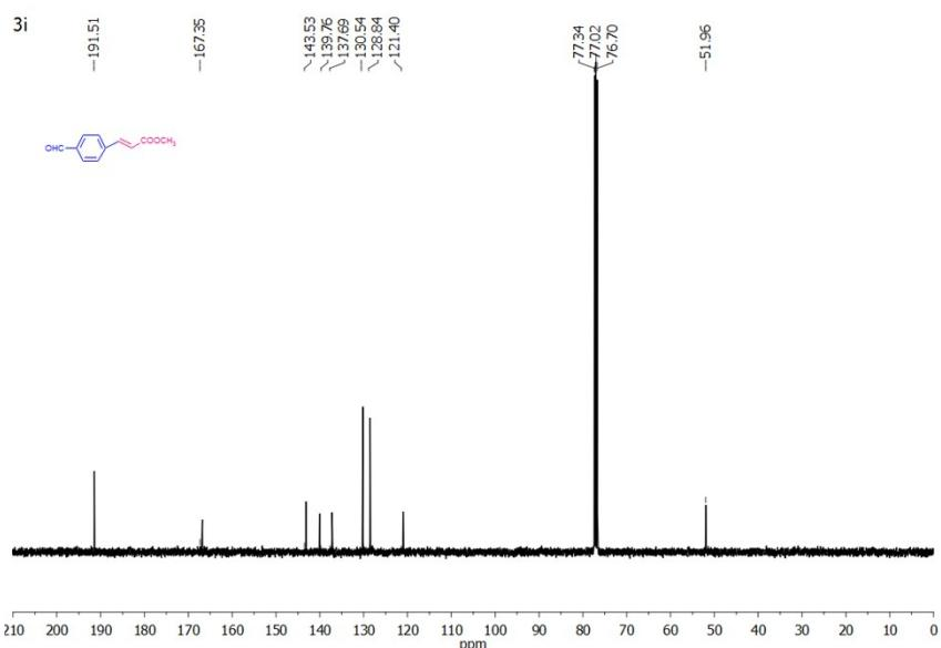
**Fig. S42:**  $^{13}\text{C}$  NMR of (E)-methyl 3-(4-formylphenyl) acrylate (3i)
