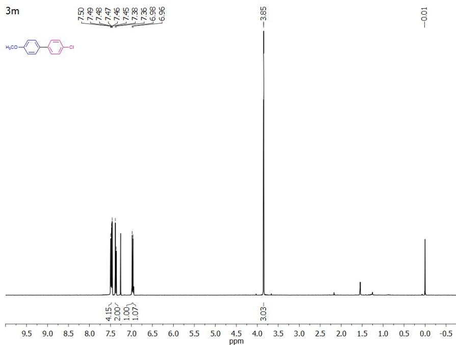
**Fig. S21:**  $^1\text{H}$  NMR of 4-methoxy-4-chloro biphenyl (3m)
