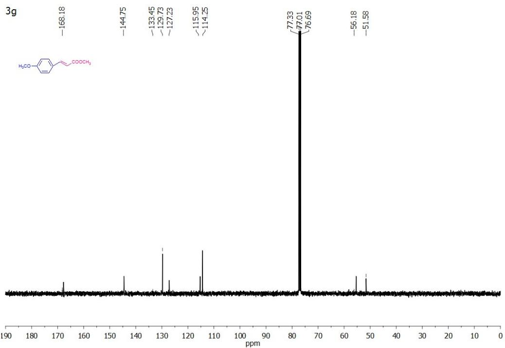
**Fig. S38:**  $^{13}\text{C}$  NMR of (E)-methyl 3-(4-methoxyphenyl) acrylate (3g)
