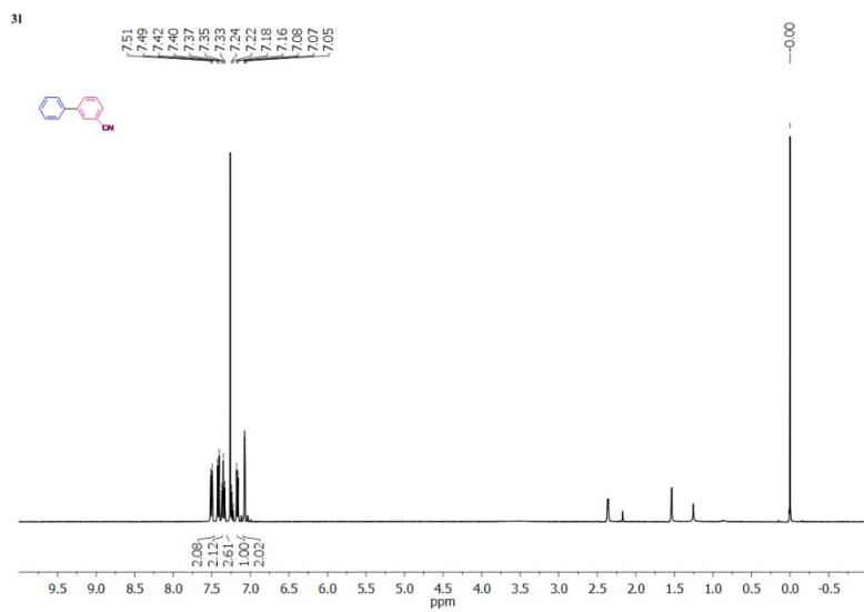
**Fig. S20:**  $^1\text{H}$  NMR of 4-cyano biphenyl (3l)
