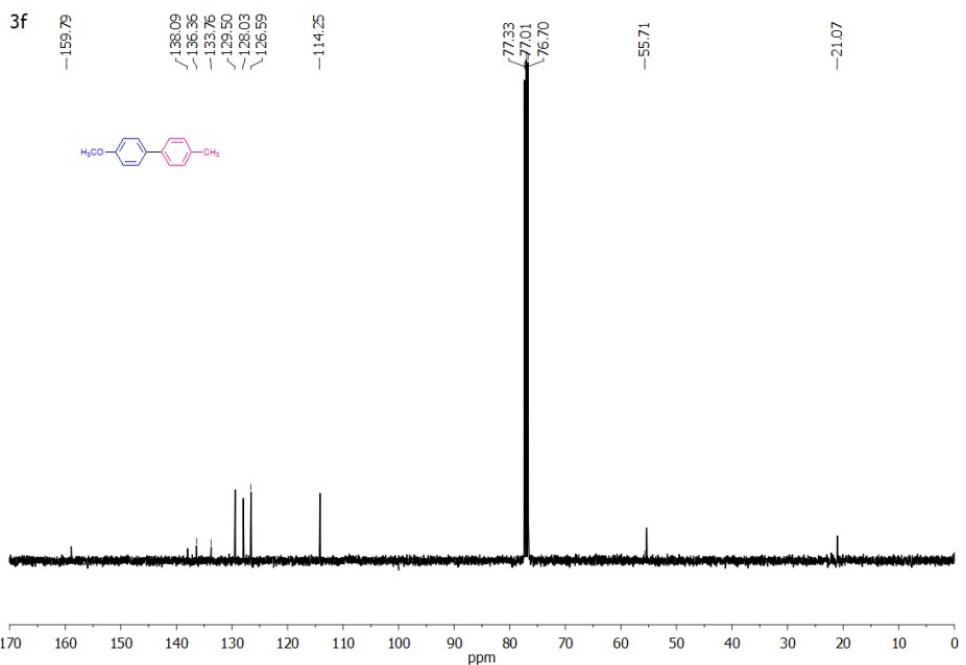
**Fig. S12:**  $^{13}\text{C}$  NMR of 4-methoxy-4-methyl biphenyl (3f)
