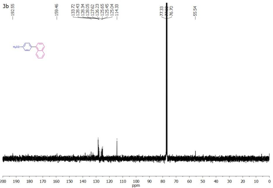
**Fig. S8:**  $^{13}\text{C}$  NMR of 4-methoxy phenyl naphthalene (3b)
