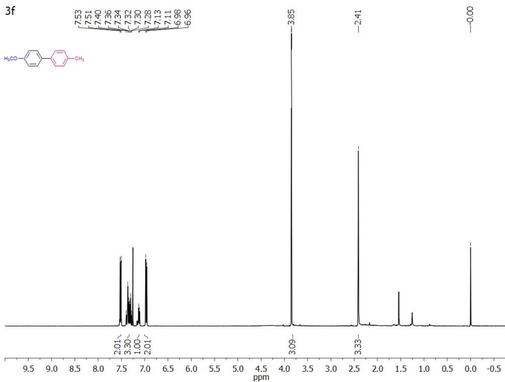
**Fig. S11:** <sup>1</sup>H NMR of 4-methoxy-4-methyl biphenyl (3f)
