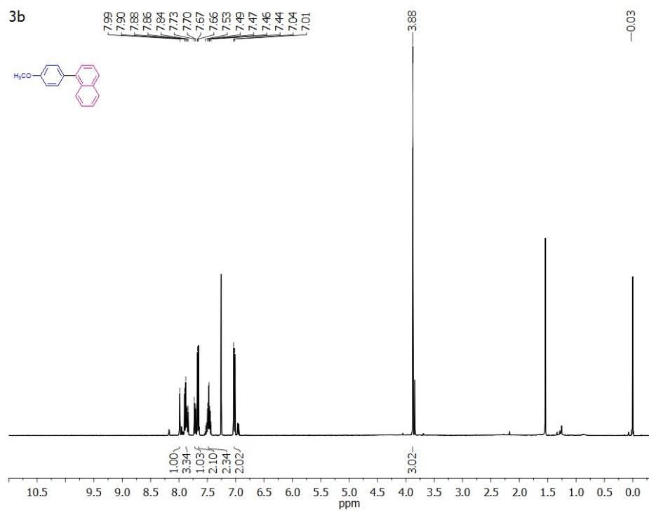
**Fig. S7:**  $^1\text{H}$  NMR of 4-methoxy phenyl napthalene (3b)
