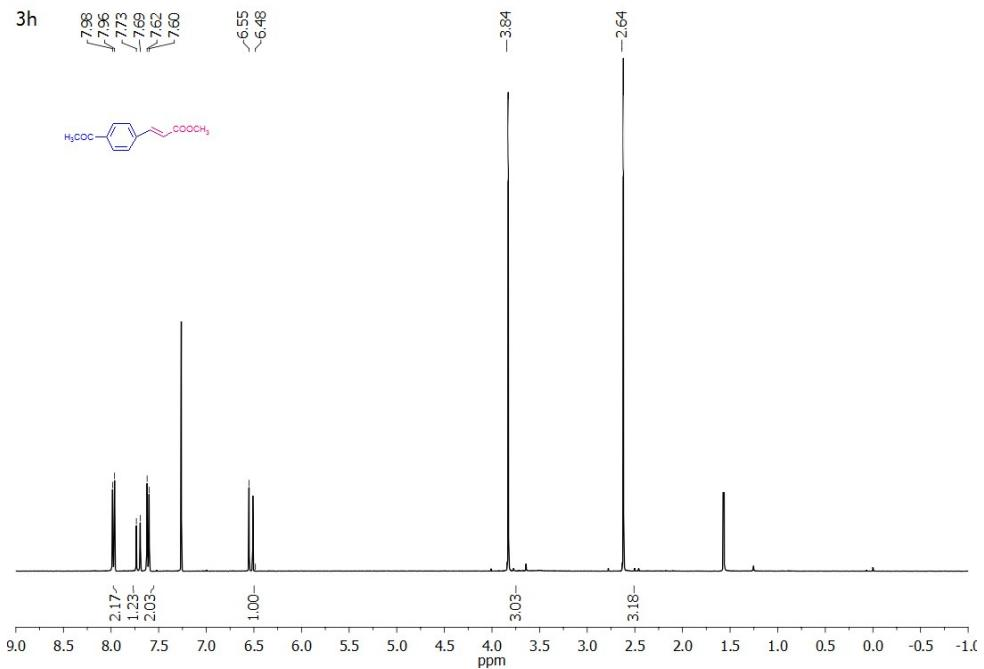
**Fig. S39:**  $^1\text{H}$  NMR of (E)-methyl 3-(4-acetylphenyl) acrylate (3h)
