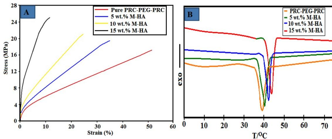
**Fig. S 1.** Mechanical strength (A) and DSC curves (B) of the M-HA/PRC-PEG-PRC nanocomposites
