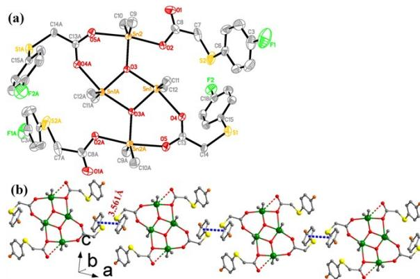
**Figure S5** The Ortep picture (a) and 1D supermolecular structure constructed by  $\pi \cdots \pi$  (blue dashes) interactions (b) of **6**. Hydrogen atoms are omitted for clarity.
