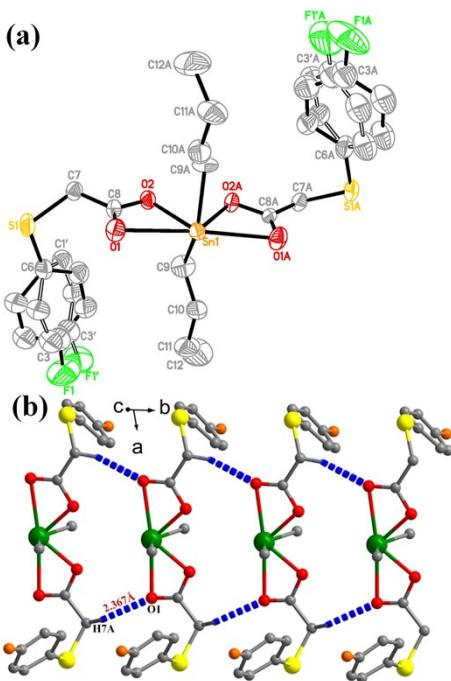
**Figure S7** The Ortep picture (a) and 1D supermolecular structure constructed by C-H $\cdots$ O (blue dashes) interactions (b) of **8**. Hydrogen atoms are omitted for clarity.
