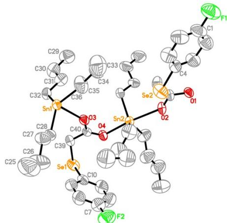
**Figure S3** The Ortep picture of **3**. Hydrogen atoms are omitted for clarity.
