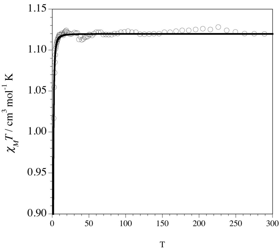
**Figure S10.** Thermal dependence of  $\chi_M T$  for **3**: (o) experimental; (—) best-fit curve through eqn (3) (see text).
