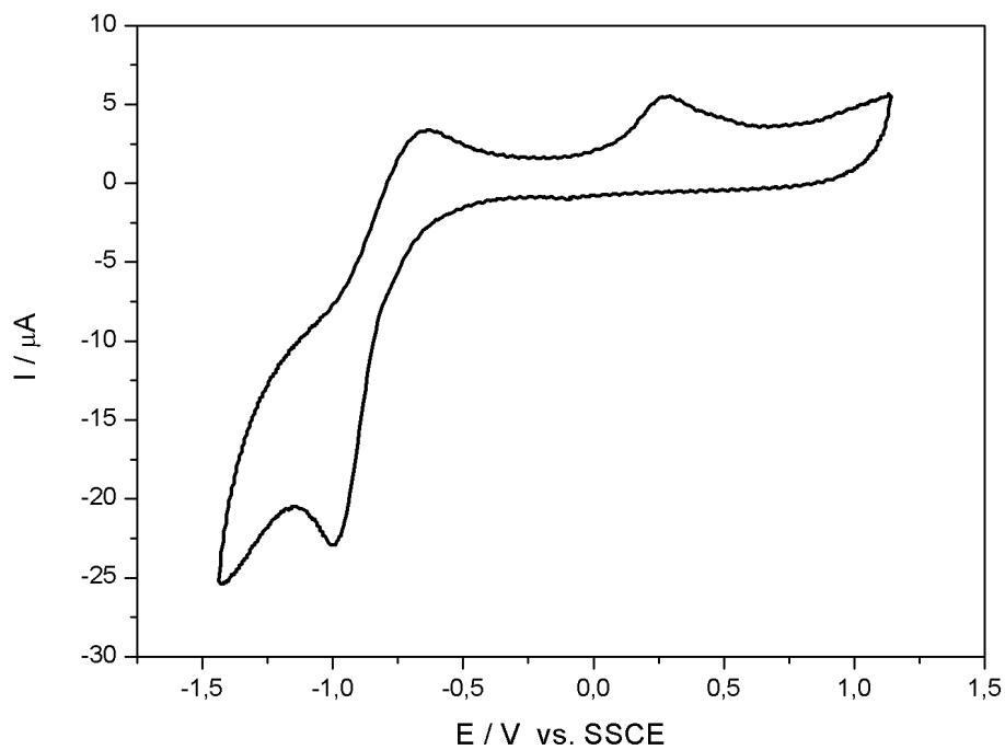
**Fig. S9** Cyclic voltammogram of **1** (0.1 M) in MeCN. Potentials are vs. SSCE, with scan rate 100 mV s<sup>-1</sup>, glassy carbon working electrode, and 0.1 M *n*Bu<sub>4</sub>NPBu<sub>6</sub>.
