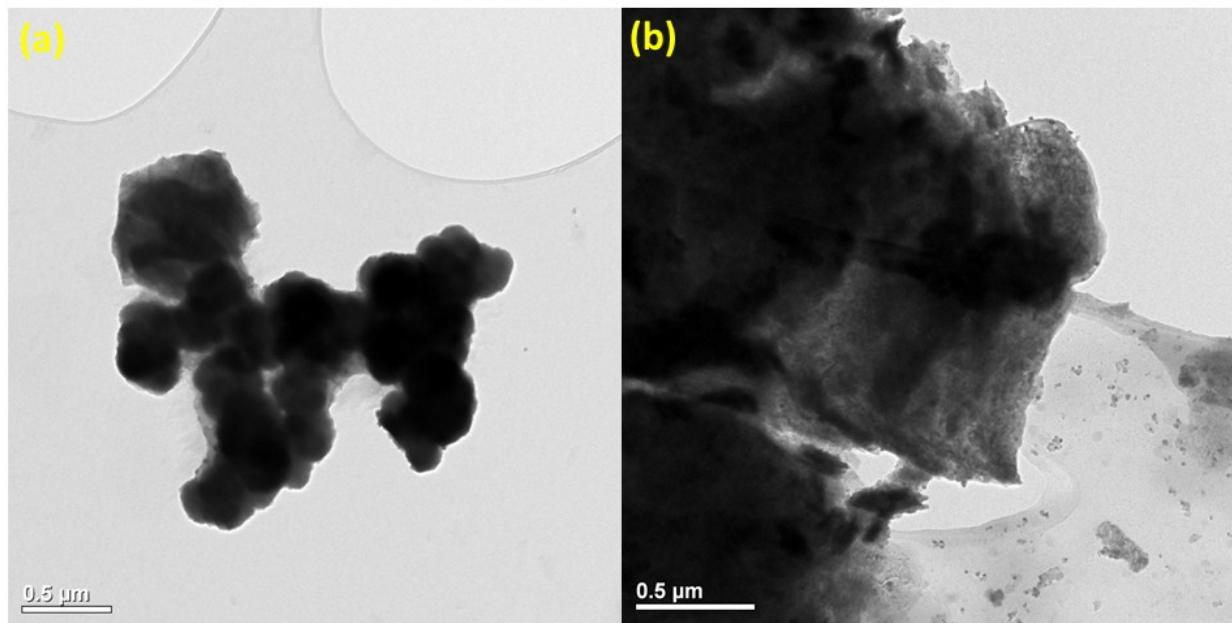
**Fig. S1** TEM images of (a) PbS/CdS/CdSe/ZnS and (b) PbS/CdS/CdSe/ZnSe sensitized TiO<sub>2</sub> film.
