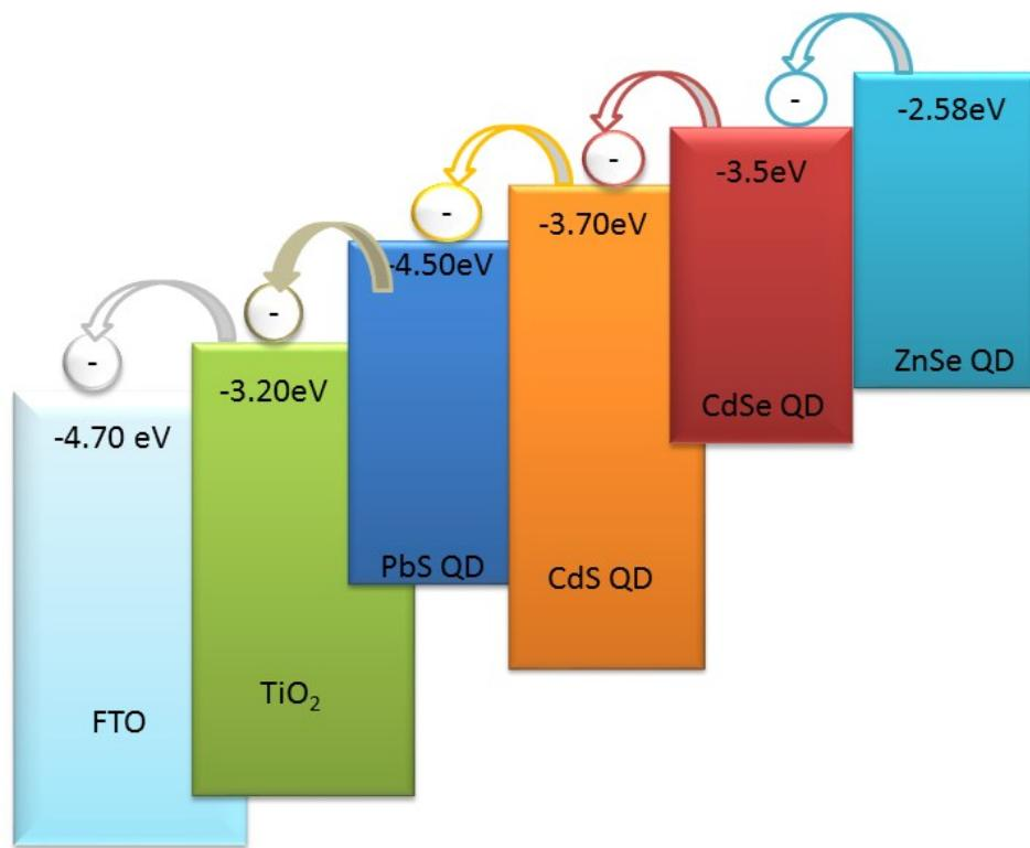
**Fig. S2** Schematic representation of the energy band gap alignment of PbS/CdS/CdSe/ZnSe sensitized  $\text{TiO}_2$  films
