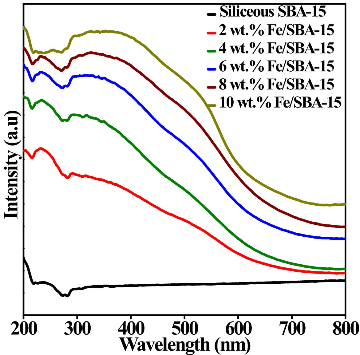
Fig.S1 DRS-UV visible spectra of SBA-15 catalysts
