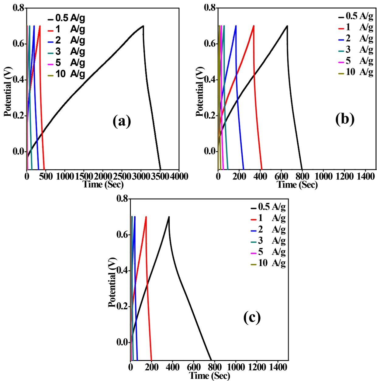
**Fig.S3** Charge-discharge profiles at different current densities of (a) NCNT 800, (b) NCNT 900 and (c) NCNT 1000.
