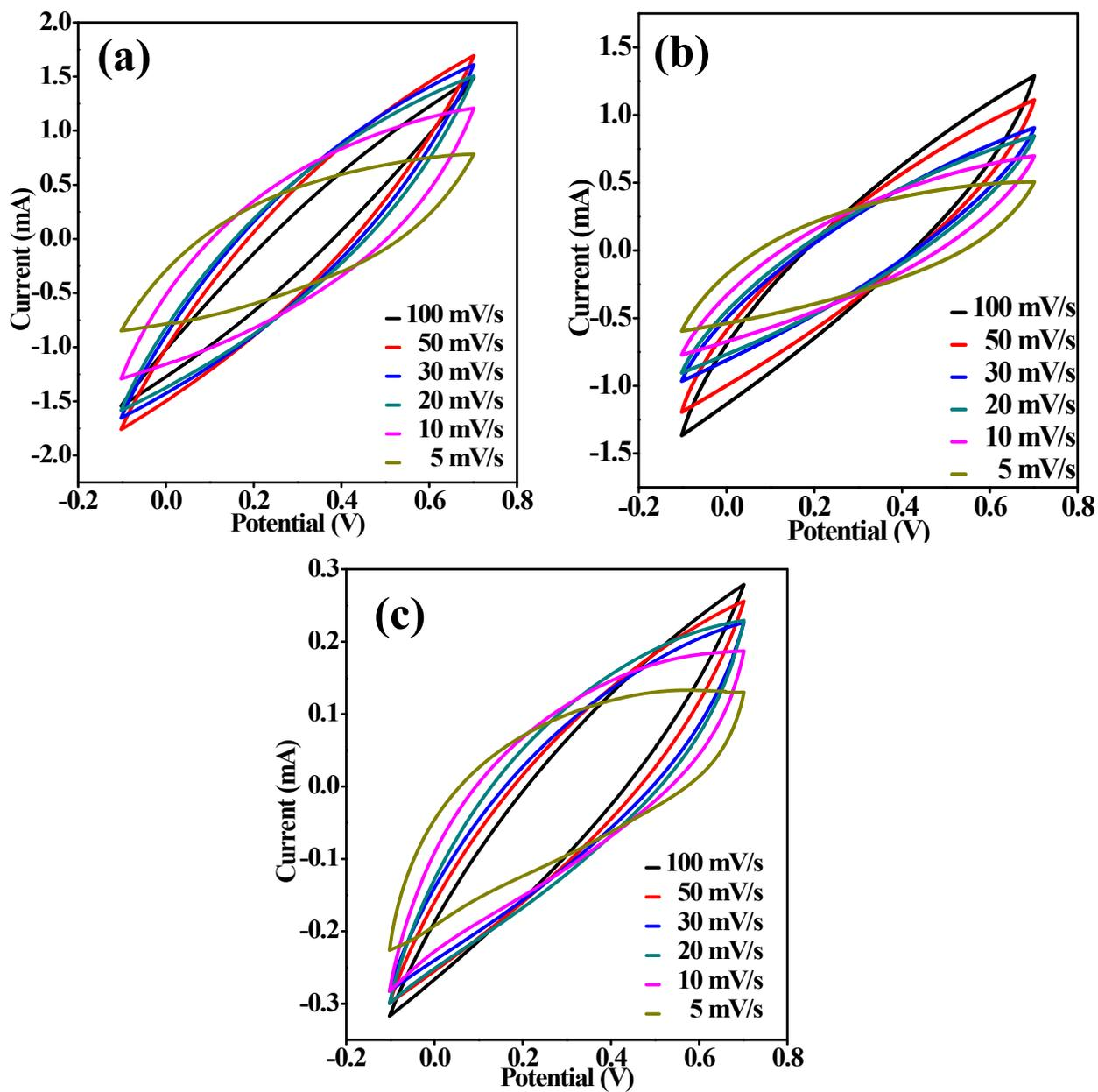
**Fig.S2** Cyclic voltammograms at different scan rates of (a) NCNT 800, (b) NCNT 900 and (c) NCNT 1000
