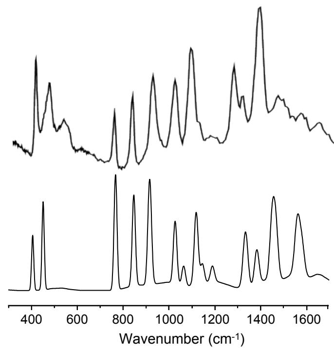
Figure S1 – Experimental INS ( $100\text{--}1650\text{ cm}^{-1}$ ) spectrum of pure 1,3-diaminopropane in the solid phase (top) and the MPW1PW/6-31G(d) calculated spectrum for the major TTTT conformer (bottom).
