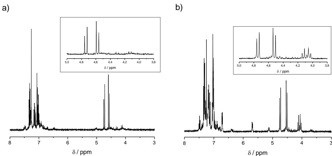
**Figure S 8** NMR spectra of compound 9 24 h after dissolution in  $\text{CDCl}_3$ . a) NMR spectrum recorded at ambient temperature and b) NMR spectrum recorded at  $-50^\circ\text{C}$ .
