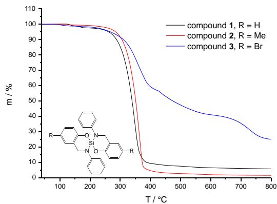
**Figure S 9** Thermogravimetric analysis of silicon compounds **1** (black line), **2** (red line), **3** (blue line); heating rate  $10\text{ K} \cdot \text{min}^{-1}$ ,  $\text{N}_2$  atmosphere,  $\text{N}_2$  volume flow of  $20\text{ ml} \cdot \text{min}^{-1}$ .
