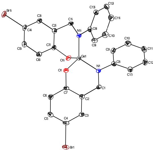
**Figure S 5** Molecular structure of **6** in the solid state (50% probability level of displacement ellipsoids, hydrogen atoms are omitted for clarity). Selected bond lengths [ $\text{\AA}$ ] and bond angles [ $^{\circ}$ ]: Ge1-O1 1.7752(17), Ge1-N1 1.801(2), O1-Ge1-O1i 108.36(12), O1-Ge1-N1 102.21(8), O1-Ge1-N1i 111.02(8), N1-Ge1-N1i 121.68(14). Symmetry transformations used to generate equivalent atoms: i denotes 2-x, 2-y, z.
