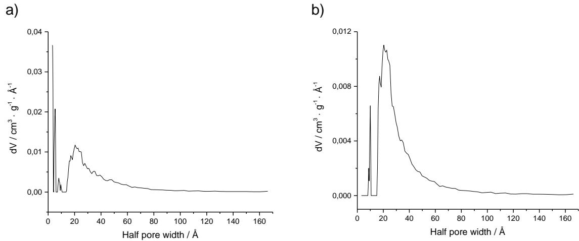
**Figure S 14** Pore size distribution of a) C4\_900 and b) C9\_900. The pore size distributions were determined according to the QSDFT model for slit and cylindrical pores using the adsorption branch for carbon materials.
