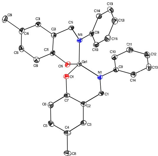
**Figure S 4** Molecular structure of **5** in the solid state (50% probability level of displacement ellipsoids, hydrogen atoms are omitted for clarity). Selected bond lengths [ $\text{\AA}$ ] and bond angles [ $^{\circ}$ ]: Ge1-O1 1.7743(12), Ge1-N1 1.8035(15), O1-Ge1-O1i 109.55(9), O1-Ge1-N1 102.74(6), O1-Ge1-N1i 110.30(6), N1-Ge1-N1i 121.06(10). Symmetry transformations used to generate equivalent atoms: i denotes 2-x, -y, z.
