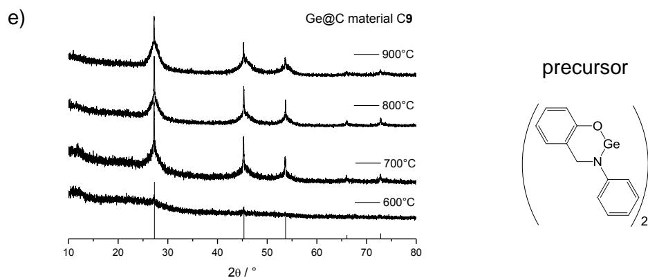
**Figure S 11** Temperature-dependent formation of crystalline germanium after carbonization of
