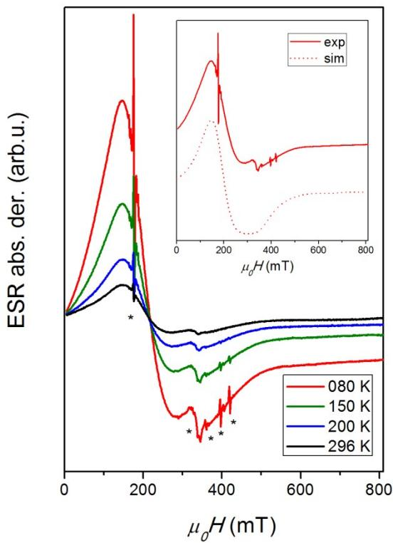
**Figure S6** ESR spectra of polycrystalline samples of **3** complex at indicated temperatures. Inset shows experimental (solid line) and simulated spectrum (dotted line) at 80 K. The spin-Hamiltonian parameters used in the simulation are given in the text.
