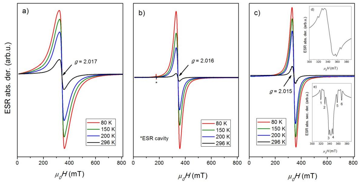
**Figure S7** ESR spectra of polycrystalline samples of a) **5**, b) **8** and c) **7** complexes at indicated temperatures. Inserts d) and e) show enlarged spectrum of **7** complex at 296 K and its derivative with labeled Mn(II) hyperfine sextet lines, respectively.
