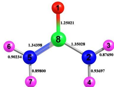
**Fig. S7.** Experimental structure of urea.
