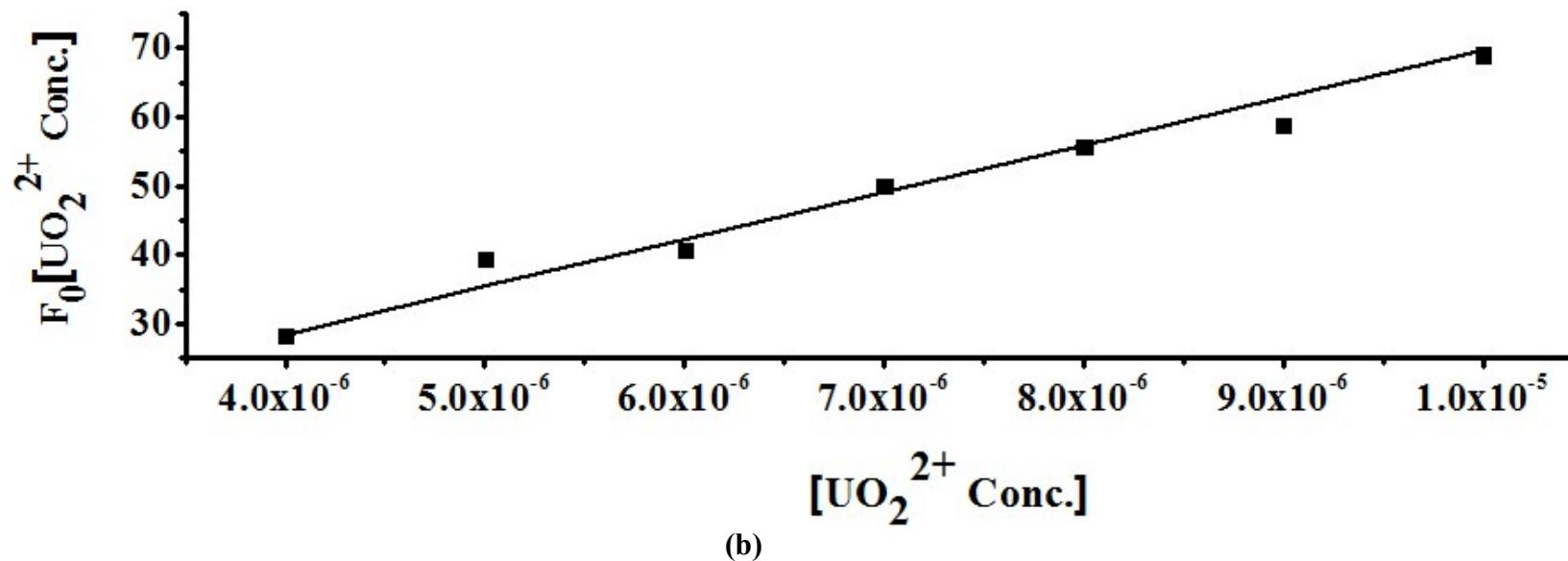
**Figure S6.** The Variation of  $E_p$  (a) with  $[\text{UO}_2^{2+}]$  concentration at fixed  $[\text{Citrate}] = 1 \times 10^{-2} \text{ M}$ ,  $I = 0.1 \text{ M NaClO}_4$  and pH 4; (b) The variation of  $F_0[\text{UO}_2^{2+} \text{ Conc.}]$  with  $[\text{UO}_2^{2+} \text{ Conc.}]$  at pH 4.
