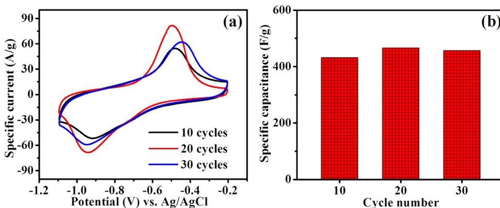
**Figure S1** Electroless cycle variation of MWCNTs/Ag electrode (a) CV curves at cycles, (b) variation of specific capacitance with different cycle number
