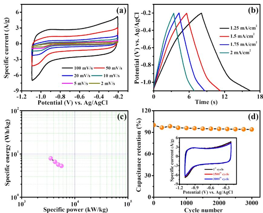
**Figure S3** Electrochemical performance of MWCNTs electrode (a) CV curves at different scan rates ranging from 2 to 100 mV/s, (b) CD curves at different current densities ranging from 1.25 to 2 mA/cm<sup>2</sup>, (c) Ragone plot related to specific energy and power, (d) Cyclic stability for 3000 cycles at 100 mV/s scan rate, inset shows CV curves for different cycle numbers
