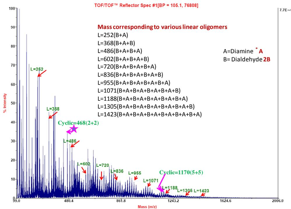
MALDI-MS of mixture of oligomers found in imine-based macrocyclisation performed for **3a** (at 0.09 M concentration)
