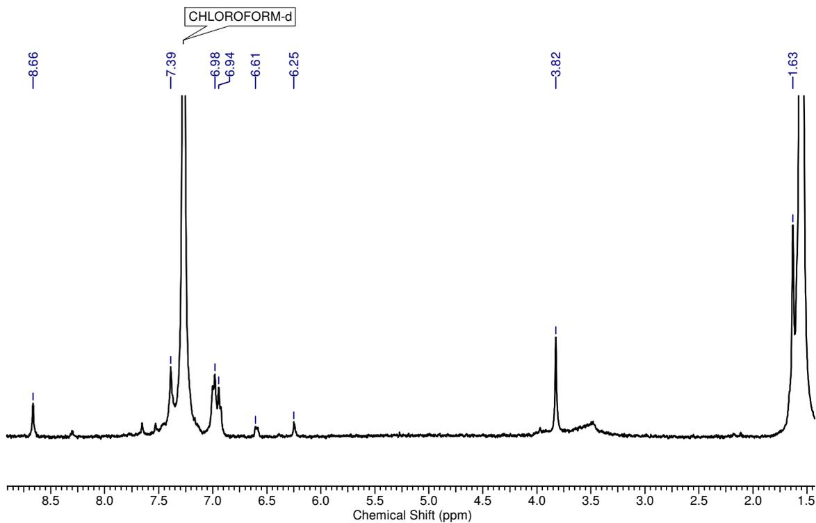
$^1\text{H}$  NMR spectrum of macrocycle **5b** ( $\text{CDCl}_3$ , 400 MHz, 298 K). *Note:* Good quality NMR spectra could not be obtained owing to the poor solubility of **5b** in  $\text{CDCl}_3$ . The peak at  $\delta=1.5$  corresponds to  $\text{CDCl}_3$ -water.
