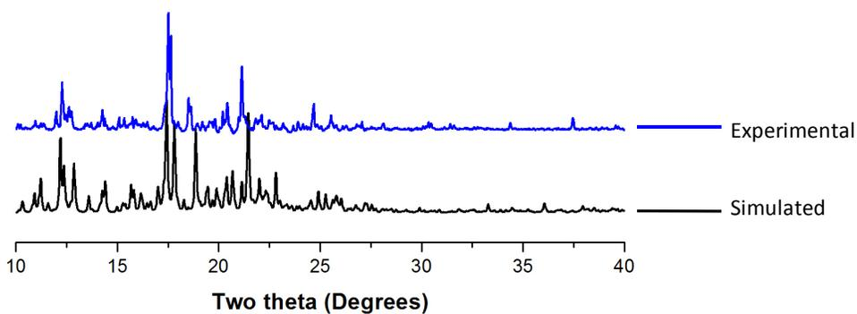
**Fig. 20** Comparison of experimental (blue) and simulated (black) PXRD (from the single crystal structure) patterns of cage **7**.
