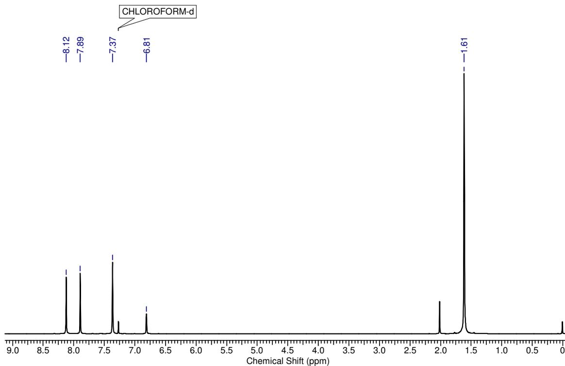
$^1\text{H}$  NMR spectrum of cage **7** ( $\text{CDCl}_3$ , 400 MHz, 298 K)
