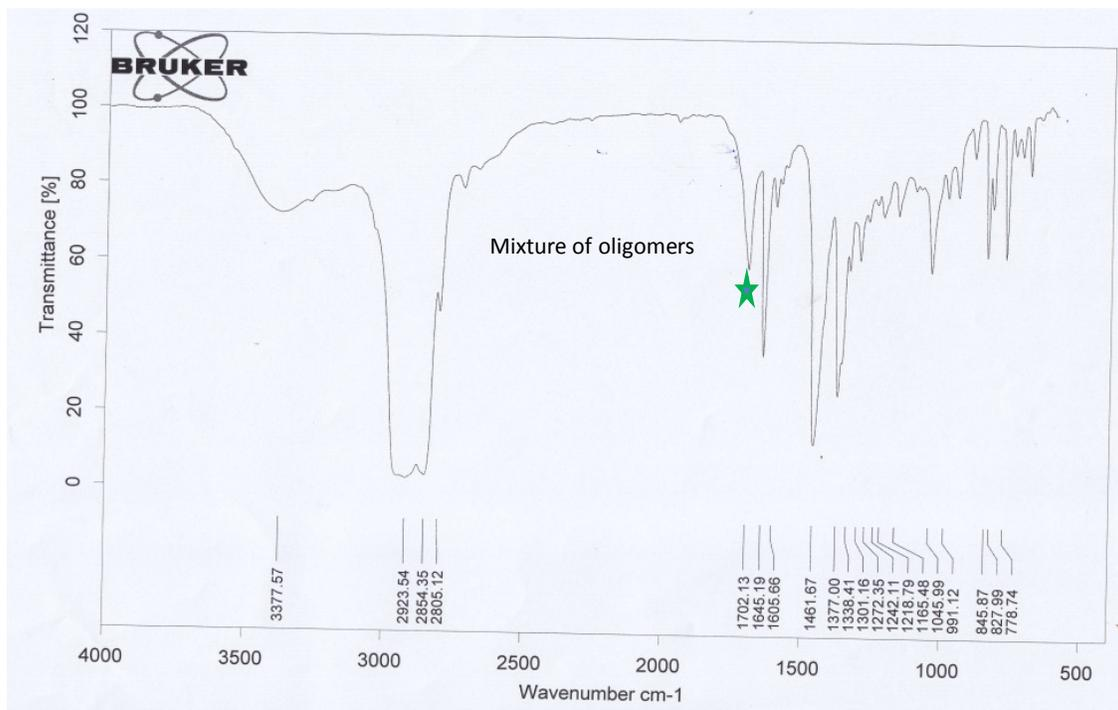
IR spectrum of imine-based macrocyclisation performed for **3a** (at 0.09 M concentration)
