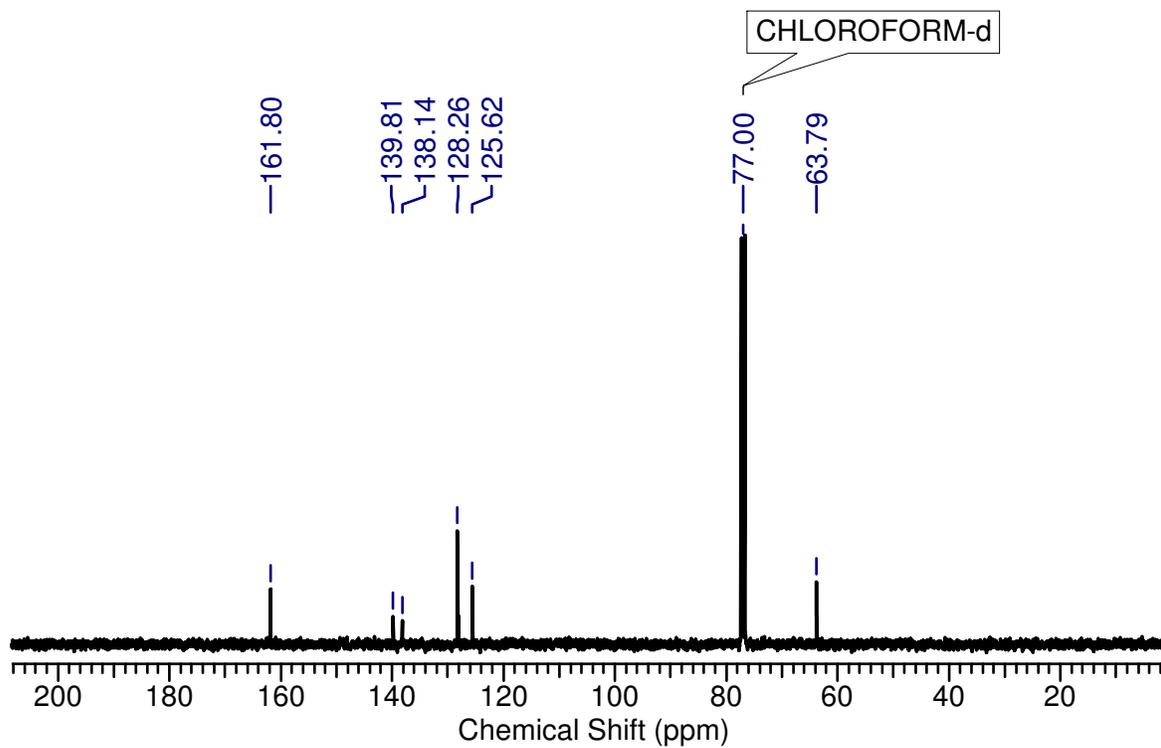
$^{13}\text{C}$  NMR spectrum of macrocycle **3a** ( $\text{CDCl}_3$ , 100 MHz, 298 K)
