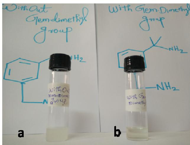
**Fig. 1** Comparison of imine-based macrocyclisation with (**1**) and without (**1a**) *gem*-dimethyl groups in the amine at 0.09 M concentration. After instant mixing of amines **1a** and **1** with dialdehyde **2a**, separately. a) Instantly formed precipitate in macrocyclisation of **3a** b) Clear solution formed in macrocyclisation of **3**.
