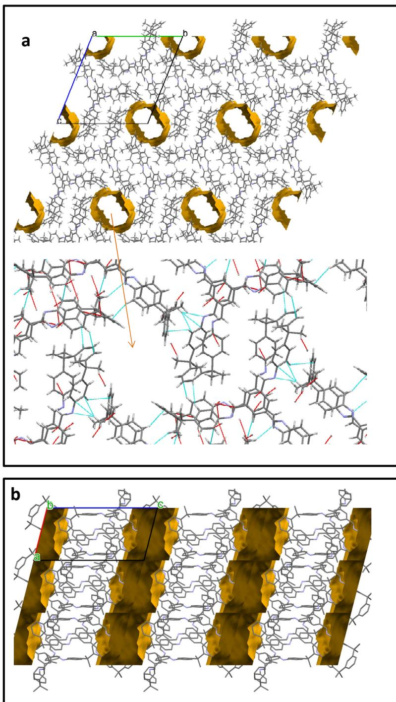
**Fig. 15** a) The successive association (through C-H...N, marginal C-H...π and other Van der Waals forces.) of six propeller-shaped cage **10** constitutes the hexagonal one-dimensional network along the a-axis. b) The voids generated along a-axis are calculated using contact surface with the probe radius 2.0 Å revealing voids amounting to 507.18 Å<sup>3</sup> per unit cell (12.9% of the cell volume).
