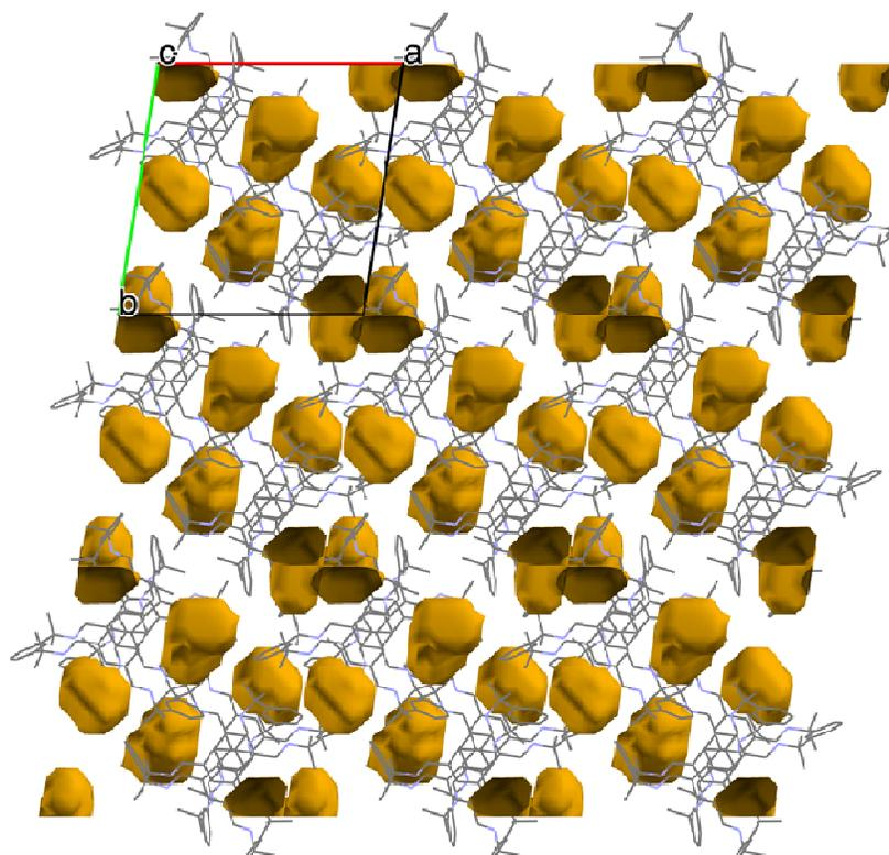
**Fig. 14** Manual deletion solvent molecules (ACN) from the crystal lattice of cage-7 generate discontinuous extrinsic voids amounting  $262.13 \text{ \AA}^3$  per unit cell (5.2% of the cell volume).
