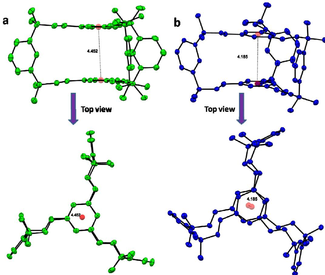
**Fig. 12** Side and top views of the two types of isomers found in the unit cell of cage-7. a) The distance between the central benzene ring is 4.452 Å and the central benzene rings were found to be in the fully-eclipsed manner, b) The distance between the central benzene ring is 4.185 Å and the central benzene rings were found to be in a slightly displaced manner.
