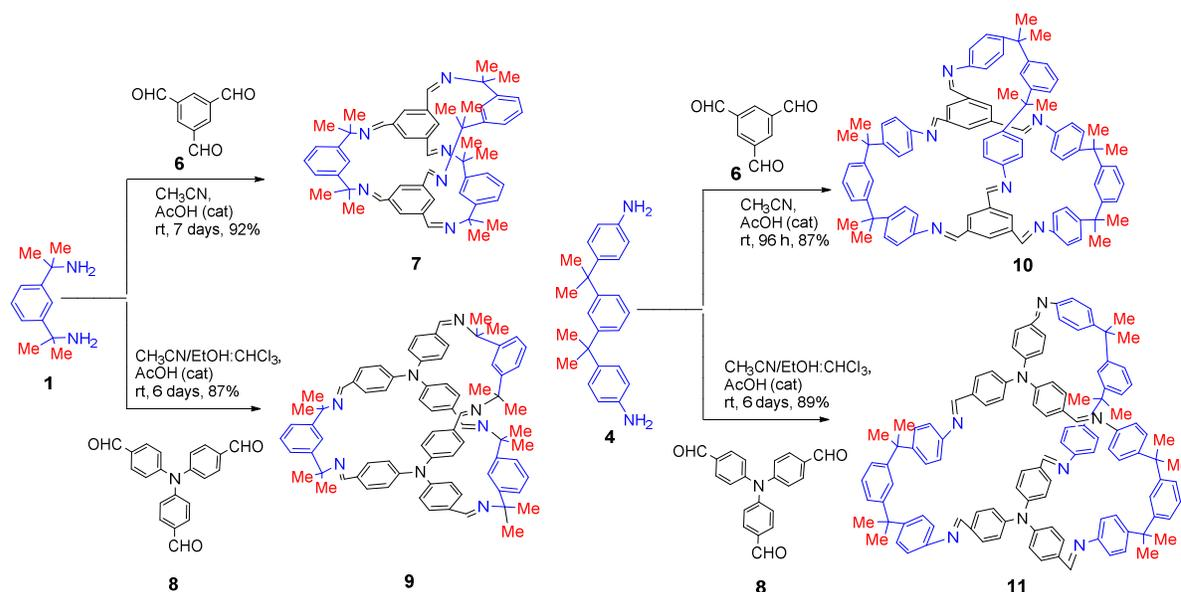
**Scheme 3:** Synthesis of cages **7**, **9** and **10** and **11** using *gem*-dimethylamines **1** and **4**.
