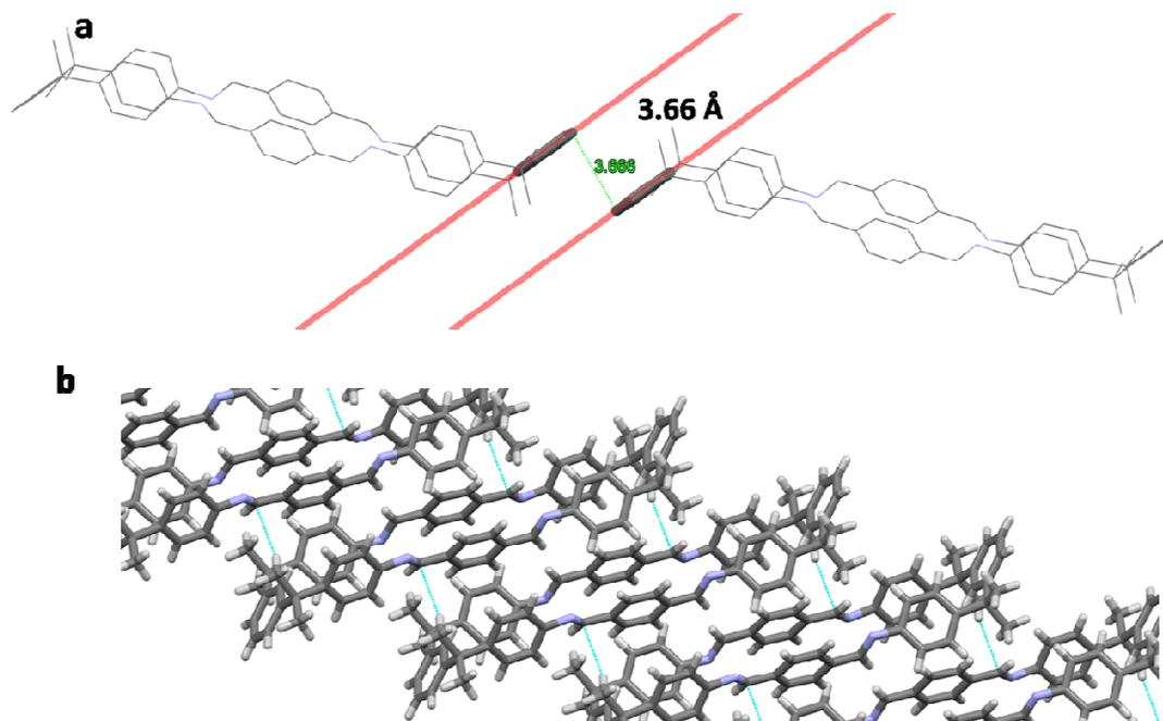
**Fig. 10** CH- $\pi$  and  $\pi$ - $\pi$  stacking interaction in the Macrocycle **5a**. a) Terminal benzene ring of the macrocycle **5a** showing intermolecular parallel displaced  $\pi$ - $\pi$  stacking with the distance of 3.6 Å. b) X-ray crystal structure of macrocycle **5a** showing continuous intermolecular CH- $\pi$  interactions.
