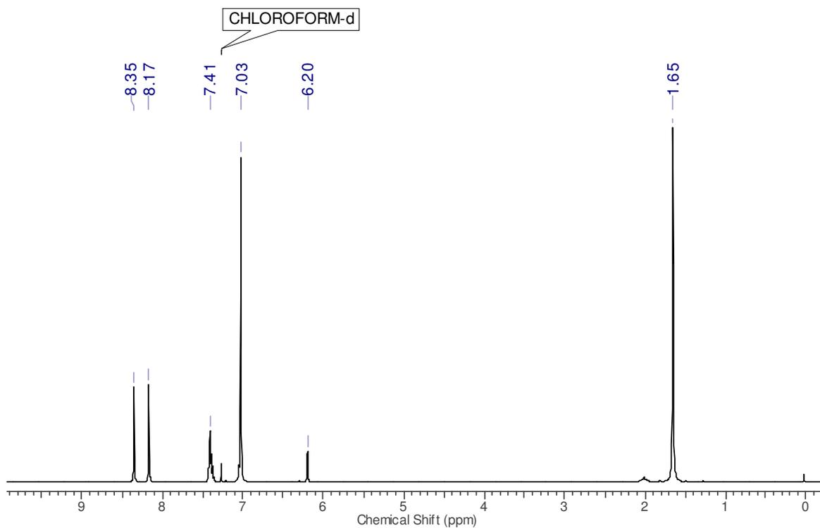
$^1\text{H}$  NMR spectrum of cage **10** ( $\text{CDCl}_3$ , 400 MHz, 298 K)
