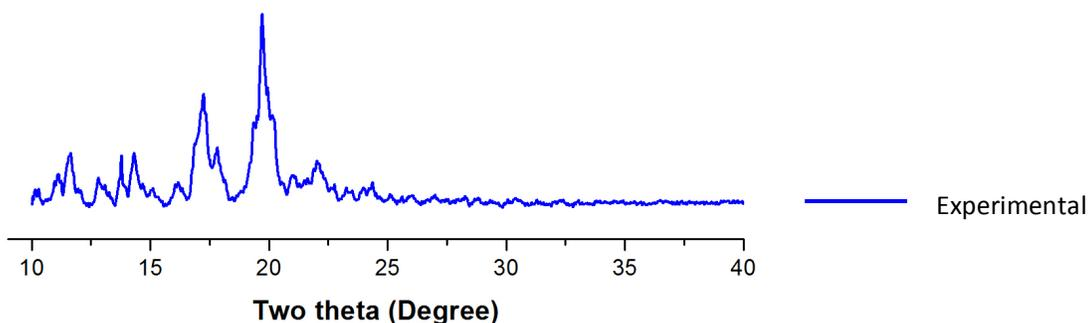
**Fig. 23** Powder X-ray diffraction pattern of cage **11**.
