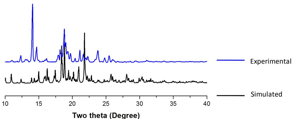
**Fig. 21** Comparison of experimental (blue) and simulated (black) PXRD (from the single crystal structure) patterns of cage **9**.
