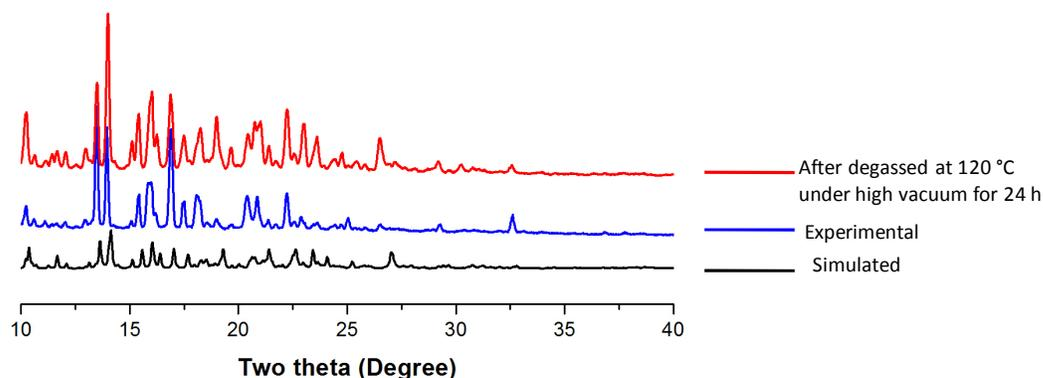
**Fig. 22** Comparison of powder X-ray diffraction patterns for **10** recorded for the bulk sample as synthesized (middle, blue), simulated PXRD from the single crystal structure for **10** (bottom, black) and after degassed at 120 °C under high vacuum for 24 h (top, red).
