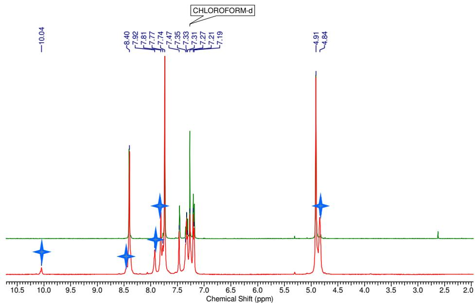
Comparison of  $^1\text{H-NMR}$  spectrum of imine-based macrocyclisation performed for **3a** at 0.09 M (red) and pure-**3a** synthesized by high dilution method (green). *Note:* Additional peaks are indicated in blue stars which correspond to other DCL).
