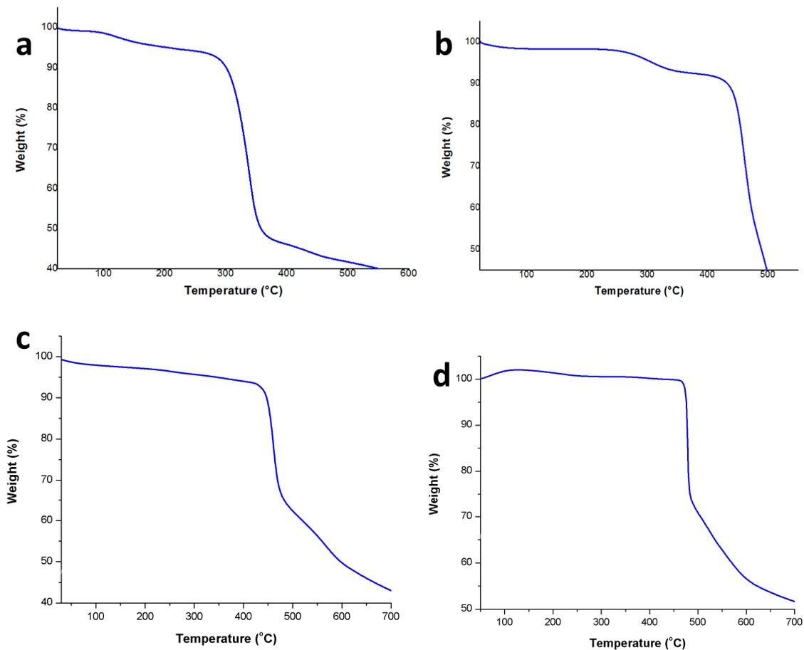
**Fig. 2** TGA data of macrocycles. a) Macrocycle-3 heated to 600 °C at the rate of 5 °C /min. b) Macrocycle-5a heated to 600 °C at the rate of 5 °C /min. c) Macrocycle-5b heated to 700 °C at the rate of 10 °C /min. d) Macrocycle-5c heated to 700 °C at the rate of 10 °C /min. *Note:* Except macrocycle-3, rest of the macrocycles showed decomposition temperature above 400 °C.
