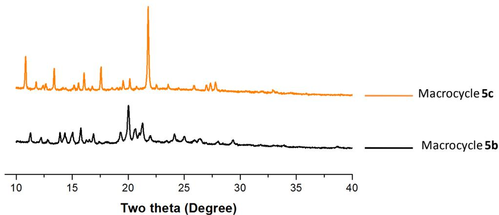
**Fig. 19** Powder X-ray diffraction patterns for macrocycle **5b** (black) and **5c**.
