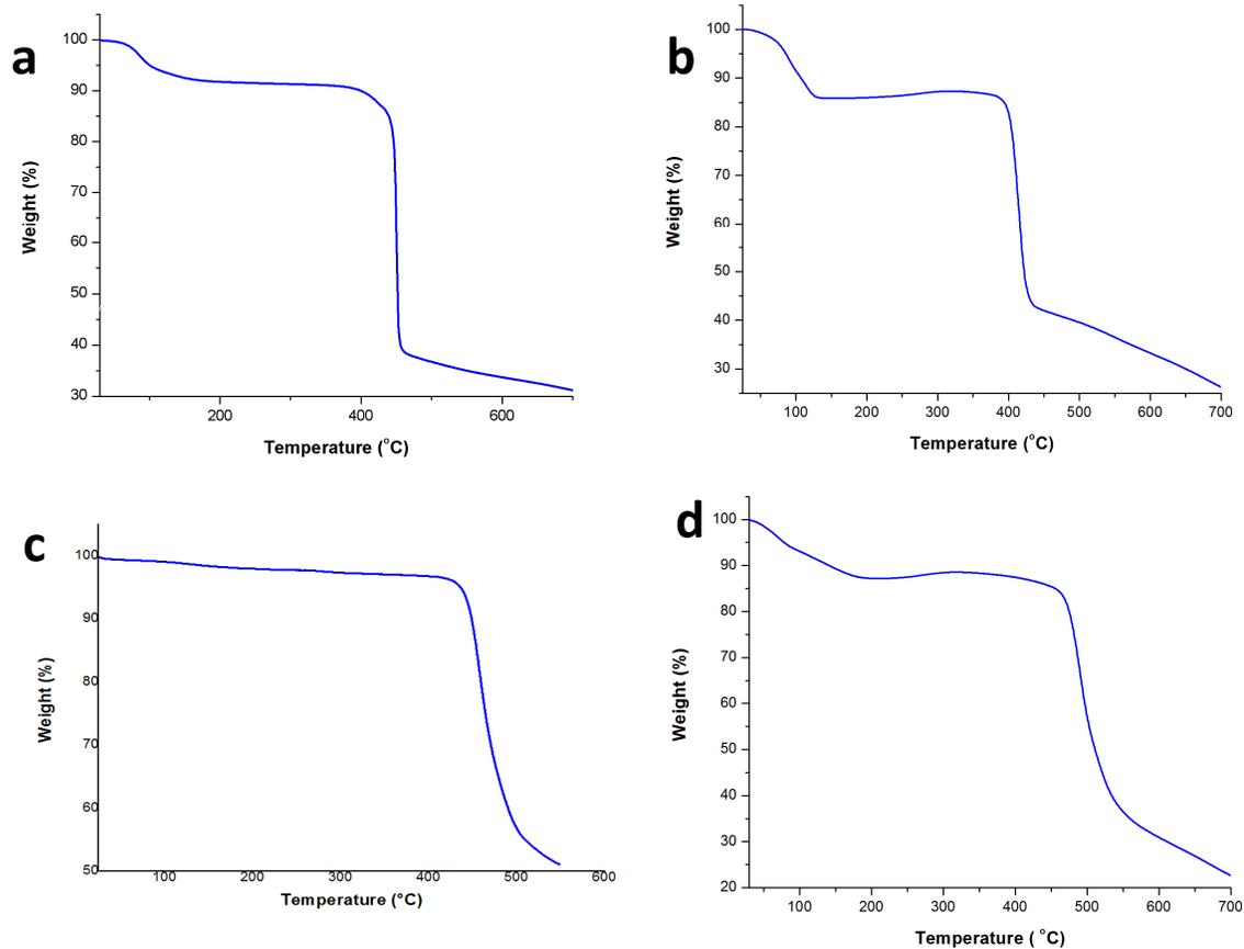
**Fig. 3** TGA data of cages. a) Cage-7 heated to 700 °C at the rate of 10 °C /min. b) Cage-9 heated to 700 °C at the rate of 10 °C /min. c) Cage-10 heated to 600 °C at the rate of 5 °C /min. d) Cage-11 heated to 700 °C at the rate of 10 °C /min.
