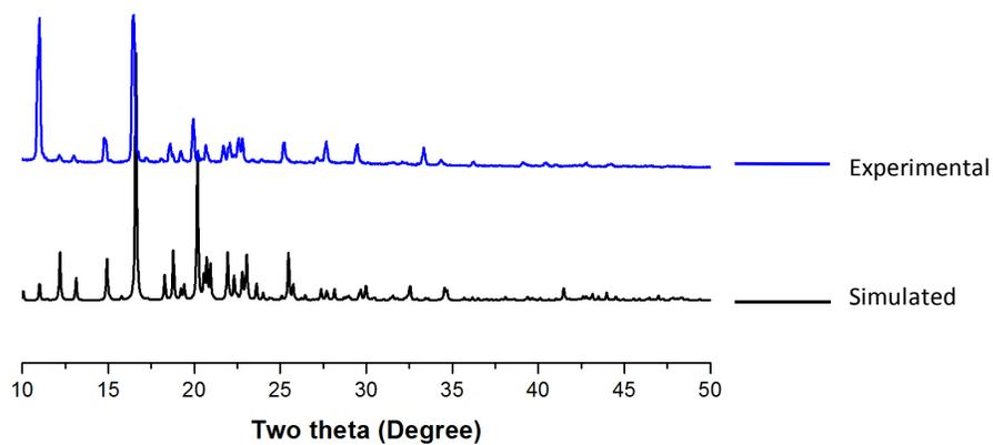
**Fig. 18** Comparison of experimental (blue) and simulated (black) PXRD (from the single crystal structure) patterns of macrocycle **5a**.
