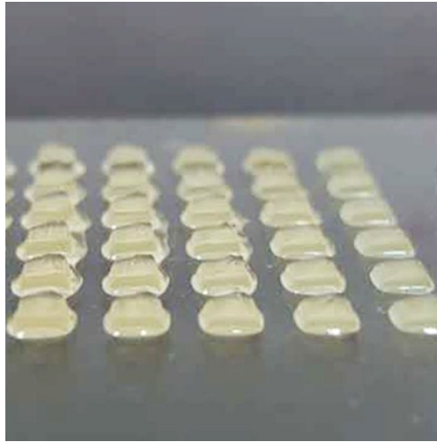
Fig. S2 Cubes array of 2mm × 2mm printed by ASIGA PICO 2 3D printer with \gamma - \text{Al}_2\text{O}_3 incorporated HDDA resins.
