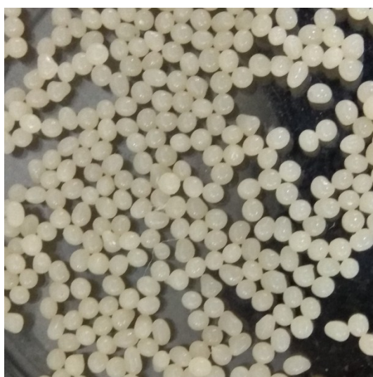
Figure S1. Gel entrapped base catalyst, Ca Alg-Base
