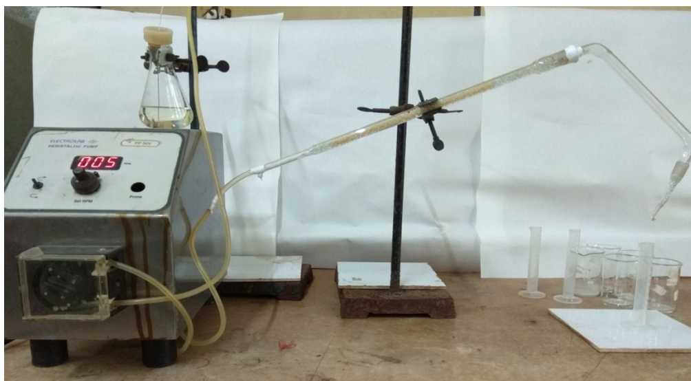
Figure S3. Set-up used to perform the reaction in continuous flow
