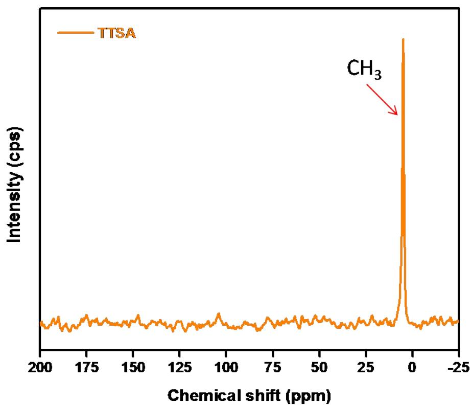
**Supplementary Figure S5**  $^{13}\text{C}$ -NMR spectrum of tris(trimethyl silyl) amine in DMSO solvent
