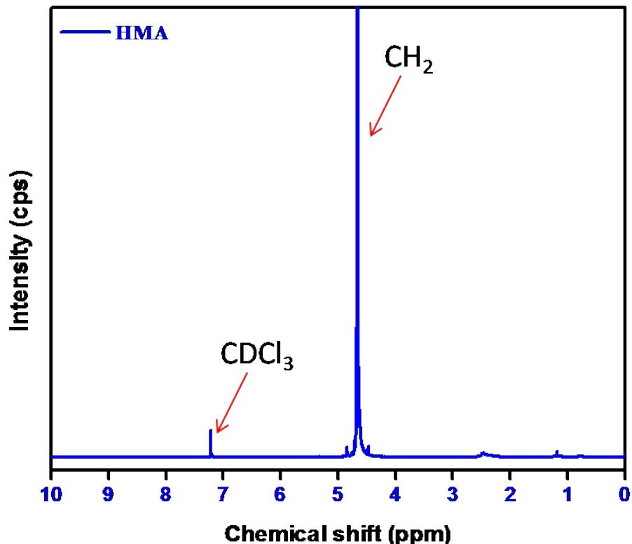
**Supplementary Figure S2**  $^1\text{H}$ -NMR spectrum of Hexamine in  $\text{CDCl}_3$  solvent
