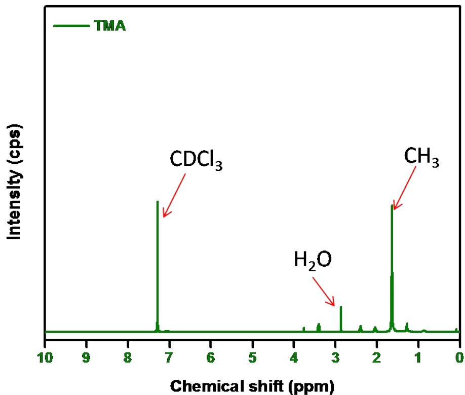
**Supplementary Figure S1**  $^1\text{H}$ -NMR spectrum of trimethyl amine (50 wt.% in water) in  $\text{CDCl}_3$  solvent
