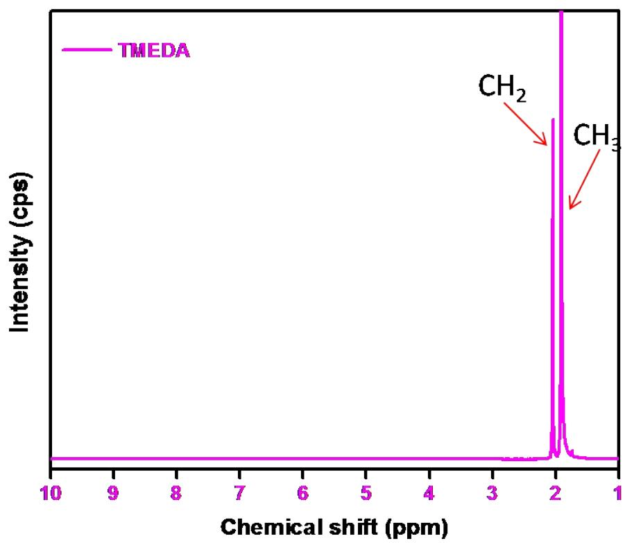
**Supplementary Figure S4** <sup>1</sup>H-NMR spectrum of N, N, N', N'- tetramethyl ethylenediamine
