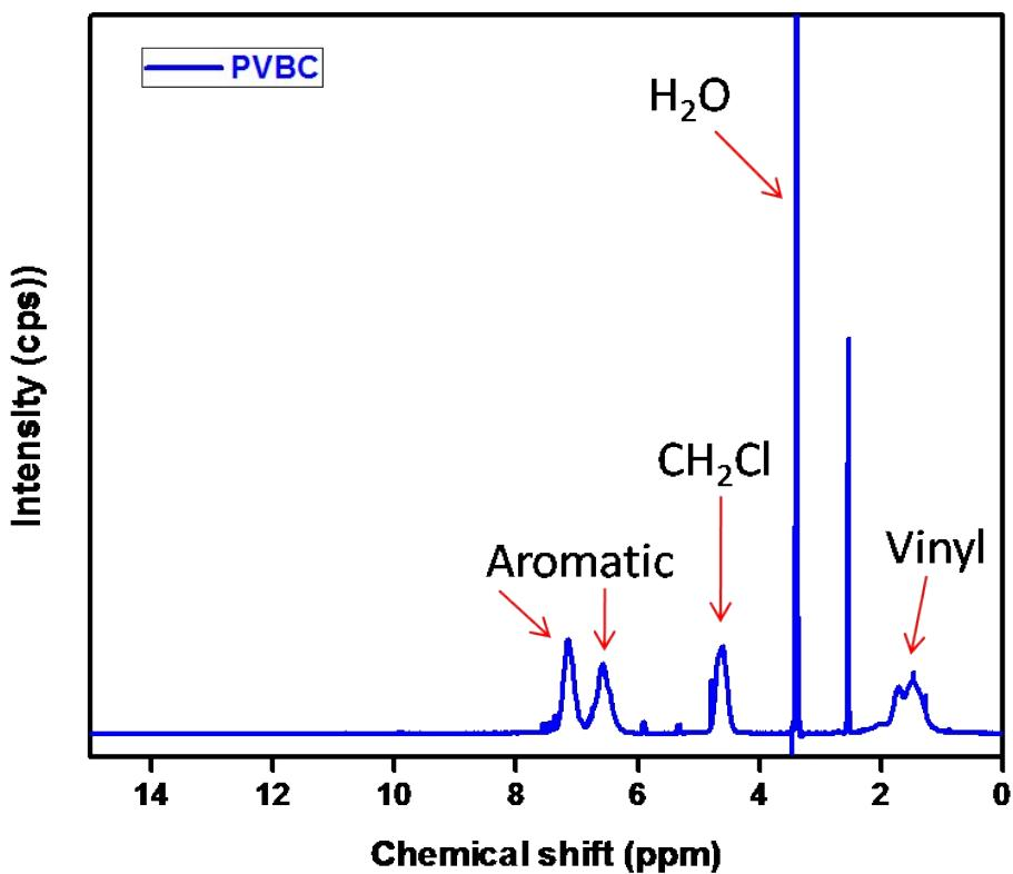
**Figure S6**  $^1\text{H}$ -NMR spectrum of poly (ST-co-VBC) polymer in  $\text{D}_2\text{O}$  solvent
