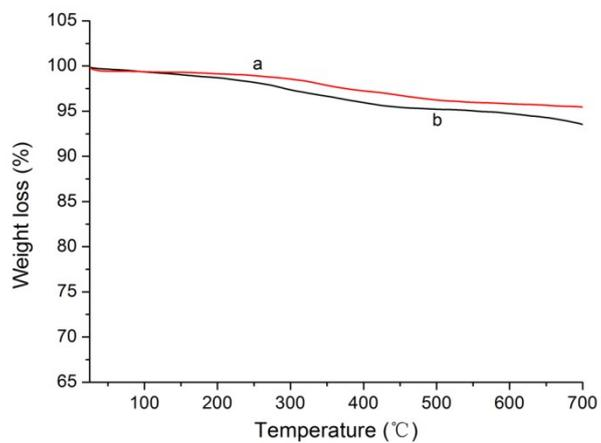
**Fig. S6** TGA curves of highly-banched Fe<sub>3</sub>O<sub>4</sub>@SiO<sub>2</sub>@Ag microflowers (a) before and (b) after six catalytic cycles.
