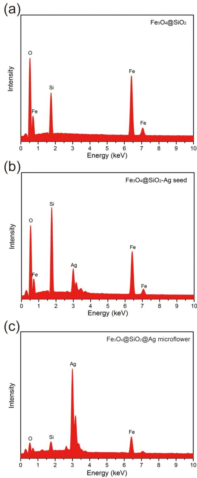
**Fig. S2** EDS spectrum of (a)  $\text{Fe}_3\text{O}_4@\text{SiO}_2$  particles, (b)  $\text{Fe}_3\text{O}_4@\text{SiO}_2\text{-Ag seed}$  and (c)  $\text{Fe}_3\text{O}_4@\text{SiO}_2@\text{Ag microflower}$ .
