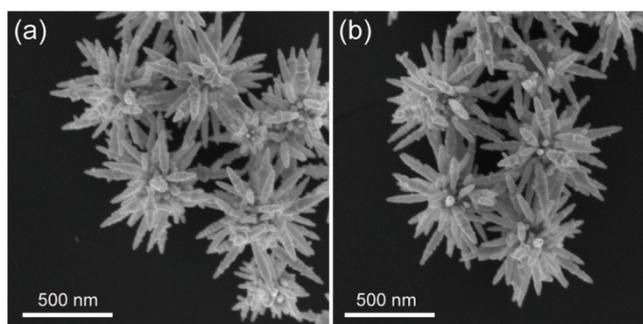
**Fig. S7** SEM images of highly-banched Fe<sub>3</sub>O<sub>4</sub>@SiO<sub>2</sub>@Ag microflowers (a) before and (b) after six catalytic cycles.
