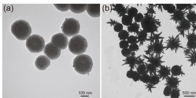
**Fig. S3** TEM images of (a) Fe<sub>3</sub>O<sub>4</sub>@SiO<sub>2</sub>-Ag seed particles with small Ag NPs (< 10 nm), (b) the corresponding Fe<sub>3</sub>O<sub>4</sub>@SiO<sub>2</sub>@Ag microcomposites. Sparse Ag petals were observed on the surface of Fe<sub>3</sub>O<sub>4</sub>@SiO<sub>2</sub>@Ag microcomposites, suggesting the too small Ag NPs on the Fe<sub>3</sub>O<sub>4</sub>@SiO<sub>2</sub>-Ag seed particles are unsuitable for the fabrication of highly branched Ag shell.
