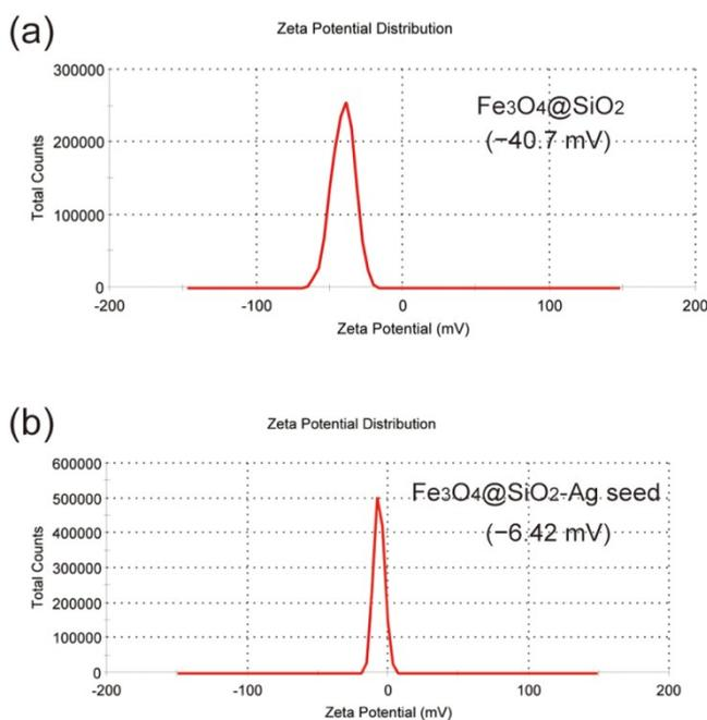
Fig. S1 Zeta potentials of (a) Fe<sub>3</sub>O<sub>4</sub>@SiO<sub>2</sub>, and (b) Fe<sub>3</sub>O<sub>4</sub>@SiO<sub>2</sub>-Ag seed particles in aqueous solution.
