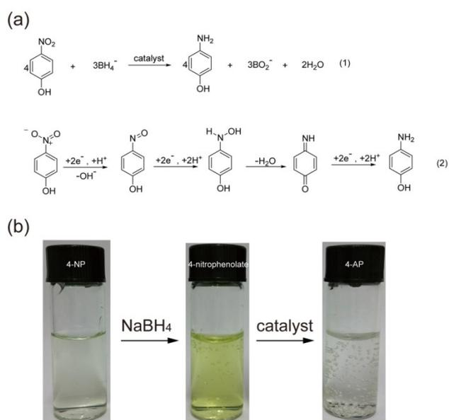
**Fig. S5** (a) The general reaction steps for reduction of 4-NP to 4-AP. (b) The change of the corresponding color in
